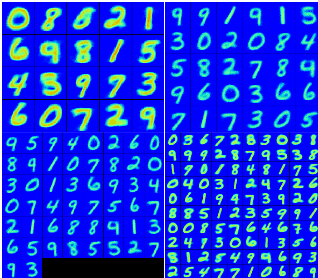
Figure 7.2: Sample heat maps of the synaptic weights after network training with four different numbers of output neurons (20, 30, 50 and 100).
