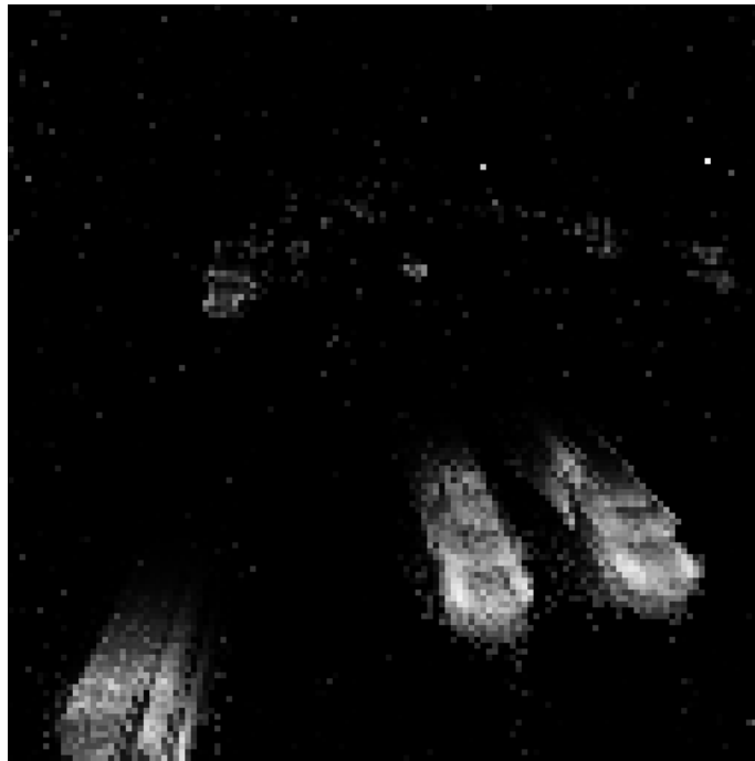
Figure 5.5: Input data for the freeway experiment coming from a spike-based camera. The spikes represent a variation of intensity for a given pixel and are generated asynchronously.
