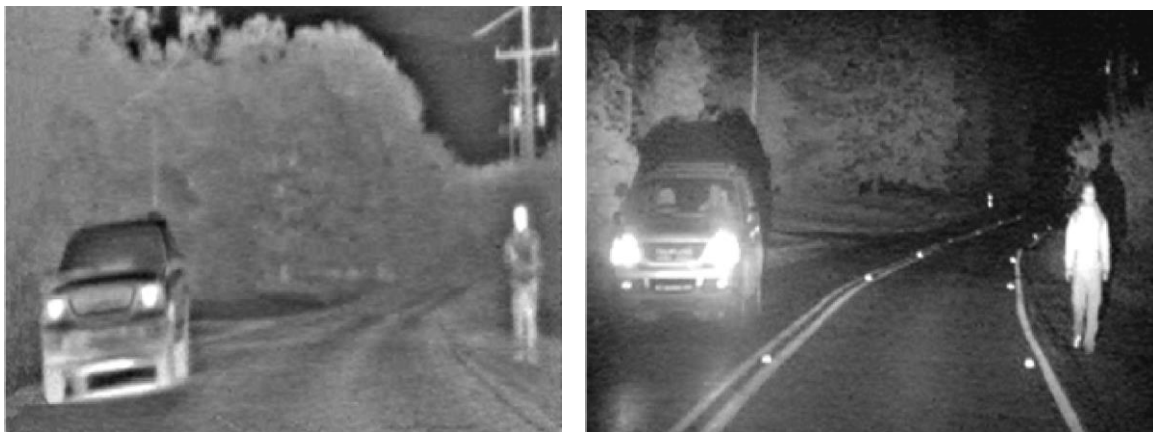
Figure 2.9. Same scene captured using an FIR-NVS (Left) and an NIR-NVS (Right) (Luo et al., 2010)
