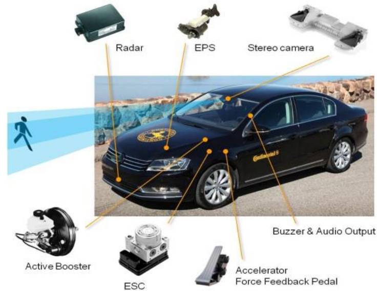
Figure 2.7. Components of a Pedestrian-CAM system (Eckert et al., 2013)
