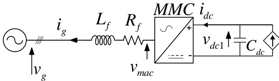
Figure 5.12 MMC connected to a variable voltage source.
