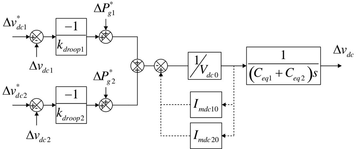
Figure 4.15 Block diagram of the equivalent HVDC link.
