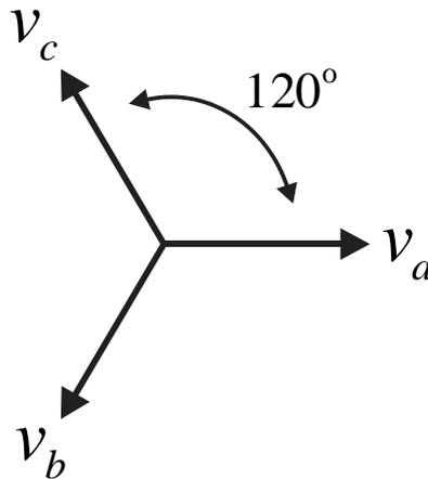
Figure 4.1 Phasorial representation of the three-phase voltage.
