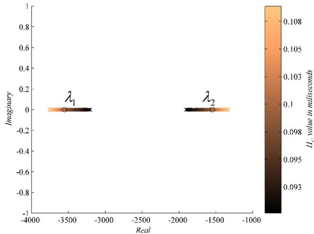
Figure 3.2 Eigenvalue trajectories for small change in  $H_C$ .
