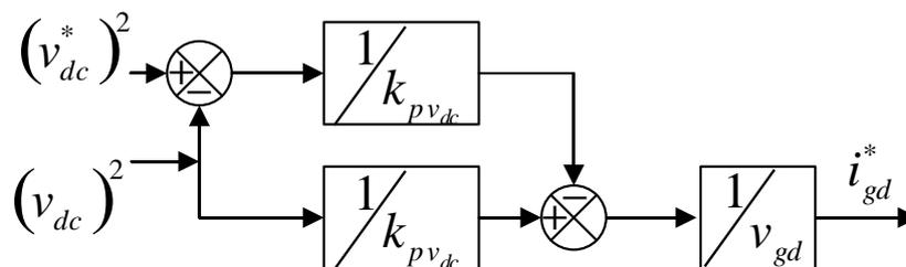
Figure 4.24  $v_{dc}$  voltage controller.
