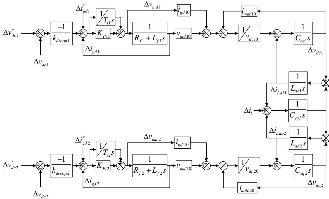
Figure 4.17 Block diagram of the MTDC system
