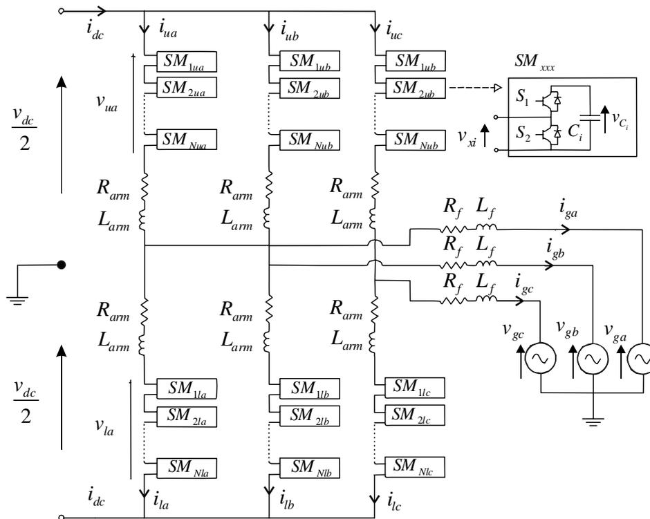
Figure 4.18 diagram of the modular multilevel converter
