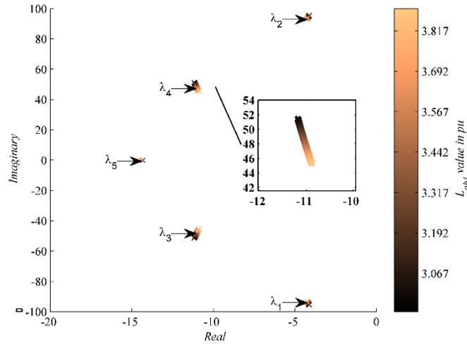
Figure 5.8 Eigenvalue evolution for changing  $L_{abl} \pm 0.5$  pu .
