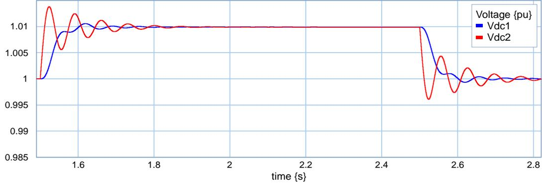
Figure 5.9 Voltage response of the VSC stations
