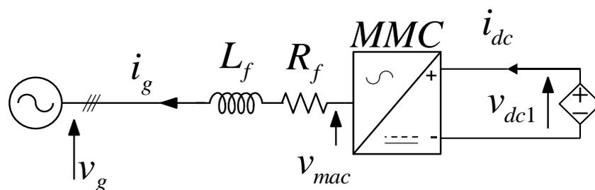
Figure 5.11 MMC connected to a fixed voltage source.
