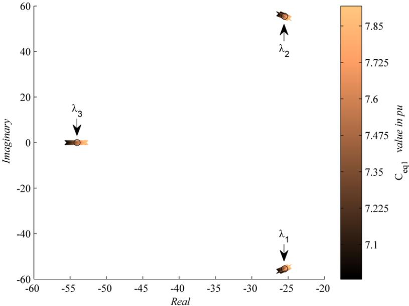
Figure 5.4 Eigenvalue trajectories changing the equivalent capacitance  $C_{eq1}$ .
