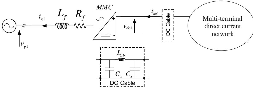
Figure 4.27 MMC station connected to a MTDC network.
