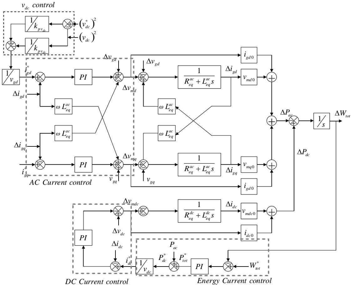
Figure 4.29 Block diagram of a voltage controlled MMC
