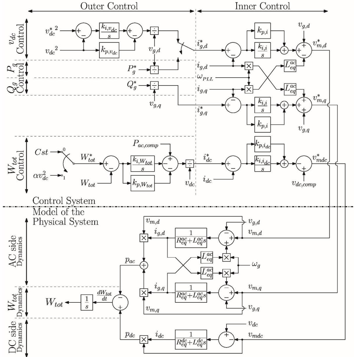
Figure 4.25 Block diagram of the complete non-linear system.
