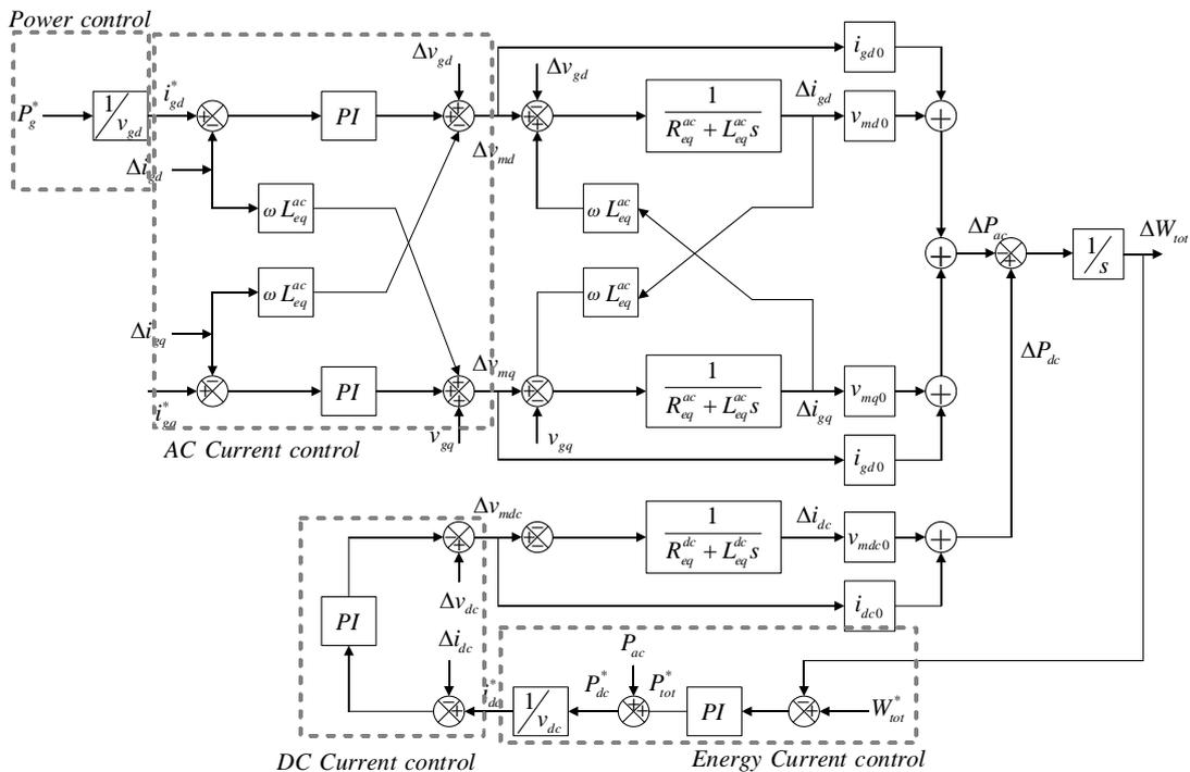
Figure 4.28 Block diagram of a power controlled MMC.
