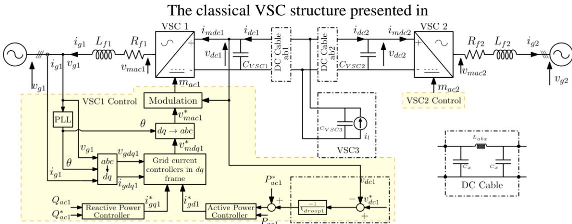
Figure 4.16 is composed of a three-phase reactor AC filter  $L_{f1}$ ,  $R_{f1}$ . The capacitor  $C_{vsc1}$ , directly connected on the DC side, is lumped in parallel with the end-point capacitor of the DC cable  $C_x$  resulting in an equivalent capacitance expressed as :
