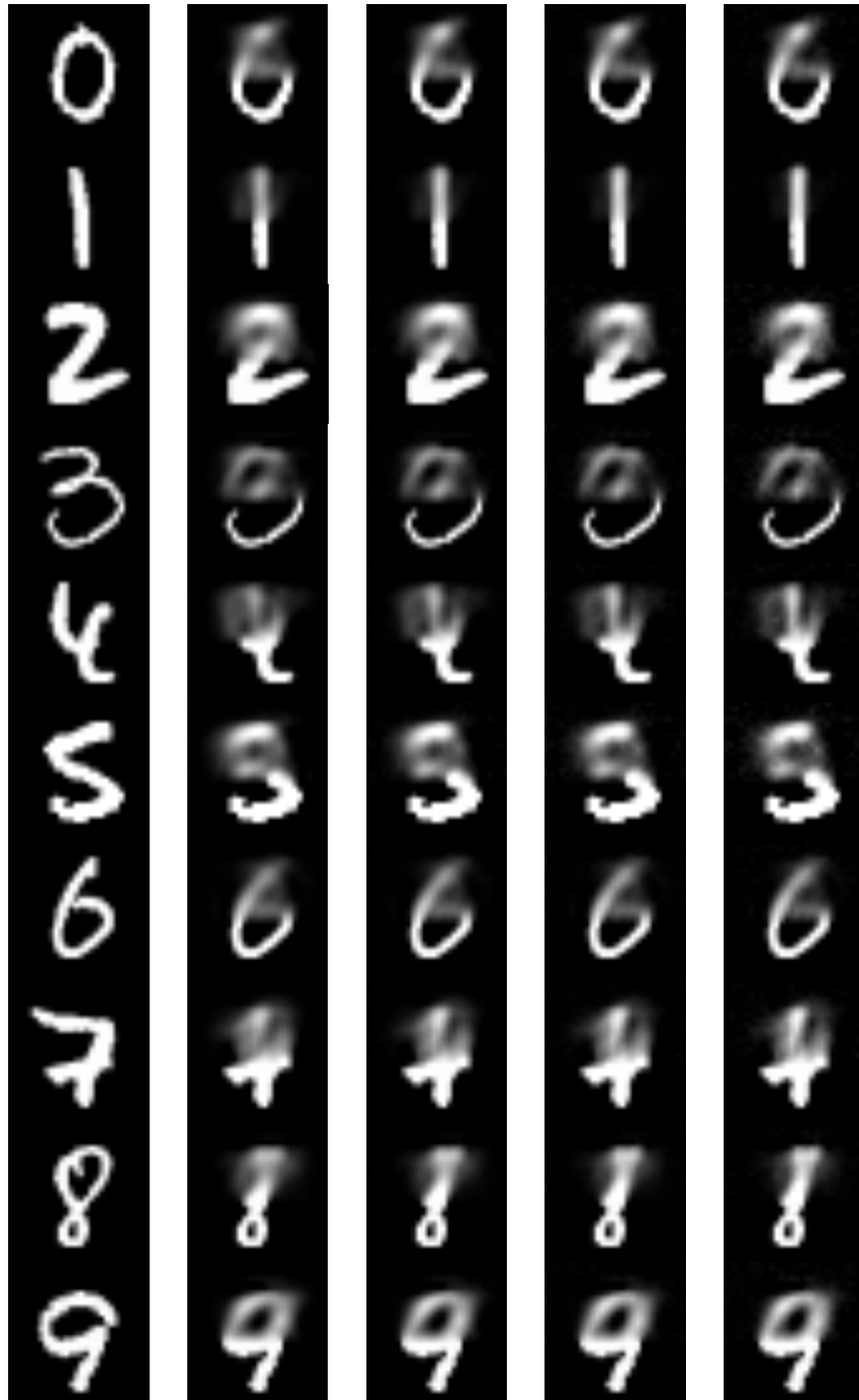
Fig. 4.4. Illustration of different loss functions for image reconstruction on MNIST. The problem is cast as a multivariate regression problem, where the top 60% pixels of the image are learned from the remaining lower 40% (i.e. \mathcal{X} = \mathbb{R}^{12 \times 28} , \mathcal{Y} = \mathbb{R}^{16 \times 28} ). From left to right we respectively display the true pixel values of 10 test images, and the pixels recovered by minimizing the \|\cdot\|_2^2 , \|\cdot\|_2^1 , \|\cdot\|_2^{0.5} and \|\cdot\|_2^{0.1} loss functions with a linear model and batch stochastic gradient-descent, i.e. tanh perceptrons. Clearly the loss function has an effect on the global consistency between the predicted pixels, with the decomposable MSE loss function \|\cdot\|_2^2 producing highly blurred images, while the \|\cdot\|_2^{0.1} loss function, closer to zero-one loss, produces less blurry images.
