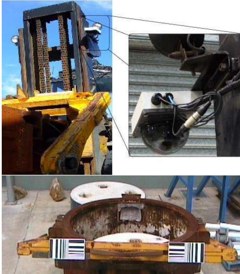
Figure 2.8: Vision setup on the hot-metal carrier. Top camera placement on top of the HMC mast, bottom camera view.
