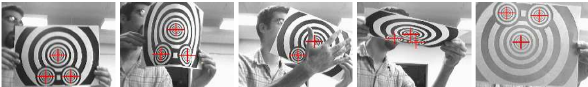
Figure 2.7: Experiment on self-similar landmark robustness, from left to right: original detection, non-rigid deformation, occlusions, perspective and loss of contrast.
