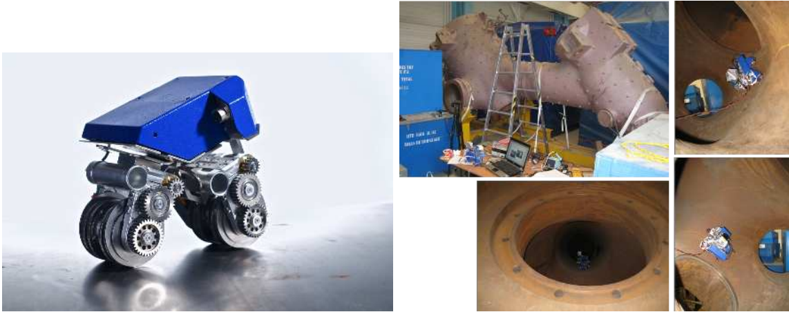
Figure 2.4: Magnebike: a robotic system to inspect metallic pipes
