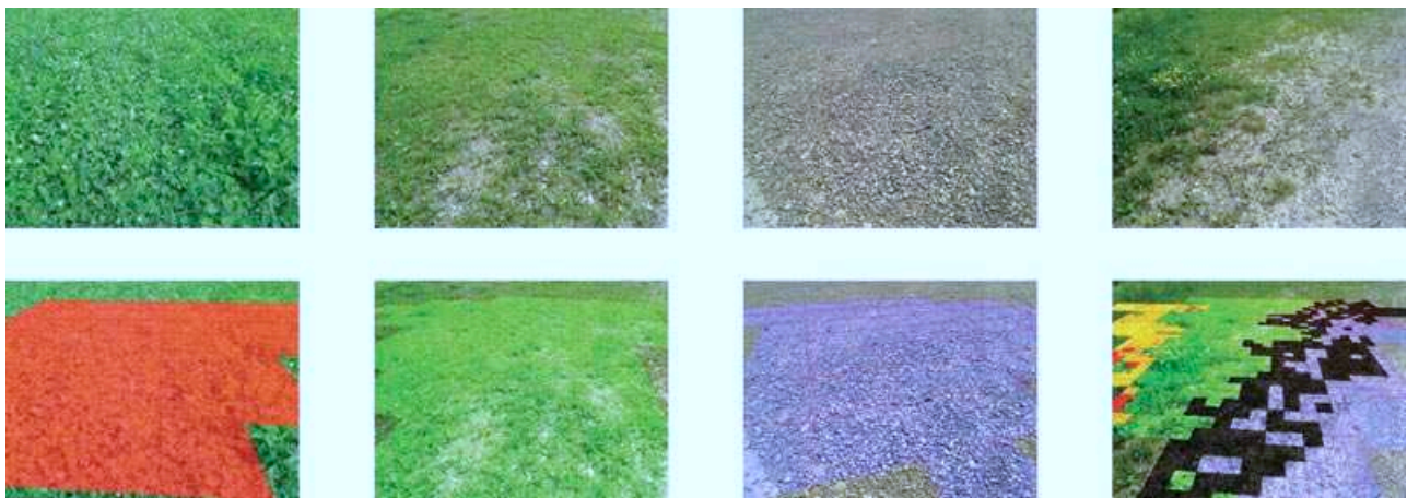
Figure 16. Typical terrains observed during the test (top) and their corresponding classification results (bottom). The overlay colors have the following meaning: red, class 1; green, 2; blue, 3; and black, 4. The class 0, or “unknown,” is in yellow (in the right-hand-side picture).
