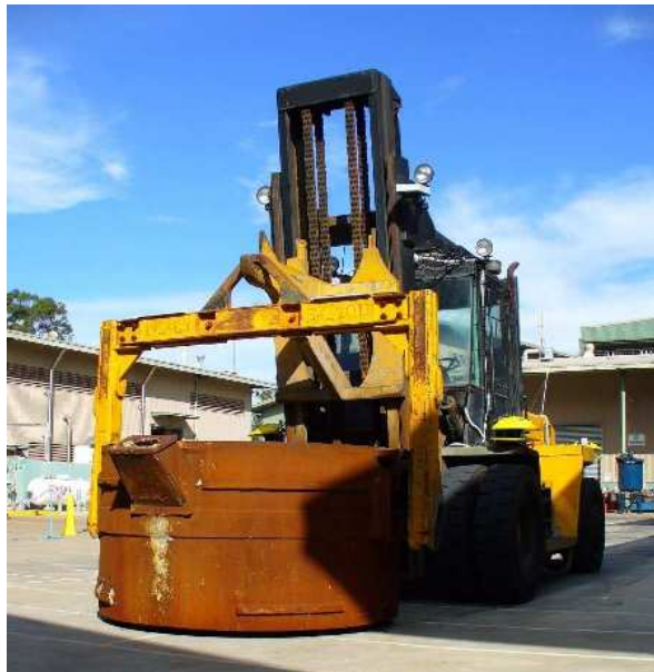
Figure 2.2: The Hot Metal Carrier, a modified forklift for the transport of liquid aluminium
