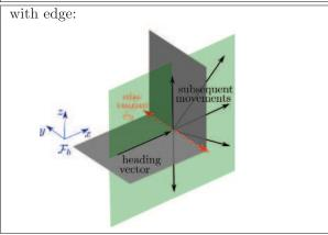
**Fig. 13.** Set of possible movement vectors  $\vec{m}_b$ , based on the robot's local frame  $\mathcal{F}_b$  for the two possible cases: (1) regular moves, where the current node is not nearby an edge; (2) edge moves, where the current node is near an edge of the environment.
