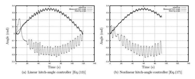
**Figure 11.** Experimental performance comparison of the linear and nonlinear hitch-angle controllers in following a sinusoidal input. Reference trajectory is shown as a solid line, actual trajectory as a dashed line, and steering angle input as a dotted line.
