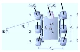
Figure 7. CRAB velocity control based on the virtual wheel. The IRC position is defined as the intersection of the middle wheels' axis and the virtual wheel axis.
