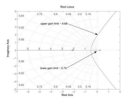
Figure 10. Root locus plot for the closed-loop system, including the steering loop dynamics, using the linear P controller.
