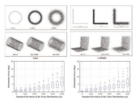
**Fig. 21.** Error in estimated orientations, predicted from tensor voting performed on a tube structure (left) and an L-shaped structure (right) as noise is varied. The results are shown in relation to the standard deviation of the Gaussian noise distribution, which was used to generate the point clouds. A few samples of the point clouds are shown above. All point clouds contain 12,000 points.
