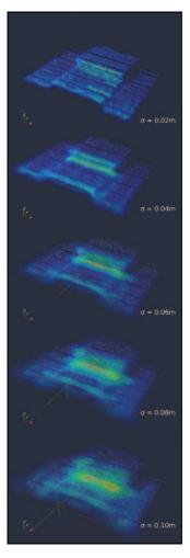
**Fig. 26.** Results of plate saliency for various  $\sigma$  values, performed on a typical lidar point cloud. This lidar scan containing 3,200 points was taken of a small metal step (see also Figure 3), approximately 6 cm high (using a Hokuyo UTM-30LX laser range finder). Surface shading represents the relative plate saliencies. The cell size used was 1 cm<sup>3</sup>. White dots show the original point cloud used for tensor voting.
