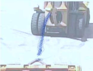
**Figure 20.** Pickup approach trajectories: superimposition of 29 pickups. The dots and the ellipse around the crucible handle show the variability of the crucible location across this set of maneuvers. The top figure shows an overview of the experiment area, and the bottom figure shows a close-up on the paths themselves. For reference, the handle width is about 2 m and the pickup hole approximately 20 cm across.
