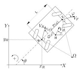
Fig. 3. Cycab robot, its landmarks and its kinematics model showing the coordinates of the flat output (point H) with respect to the reference frame of the robot placed at point F. In our case we have that  $(x_F, y_F, \theta, \varphi)$  is the state of the robot.
