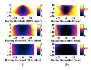
Fig. 7. Justification of the assumption for outlier rejection. (a) Bearing threshold (in rad) for a fixed inlier ratio. (b) Outlier ratio by fixing bearing threshold (in rad).
