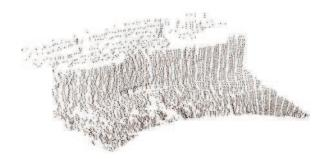
**Fig. 3.** Example of a lidar point cloud of a small metal step, which is heavily affected by noise and density variations. The point cloud contains 6,000 points, and was obtained from a Hokuyo URG-04LX laser range finder.
