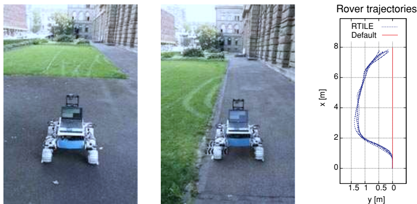
Figure 20. Test 4: CRAB rover at the starting point of first part (learning phase on the left-hand side), of the second part (middle), and resulting test trajectories (right). The traces left by the rover in the grass during the previous trial can be observed.
