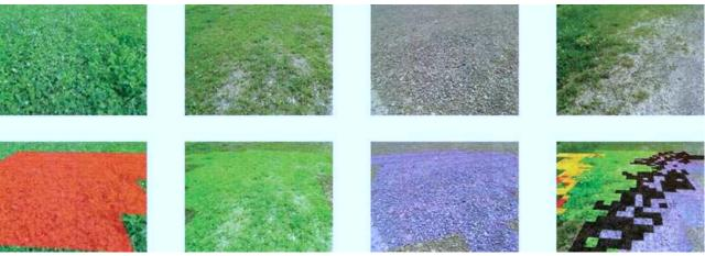
**Figure 16.** Typical terrains observed during the test (top) and their corresponding classification results (bottom). The overlay colors have the following meaning: red, class 1; green, 2; blue, 3; and black, 4. The class 0, or "unknown," is in yellow (in the right-hand-side picture).
