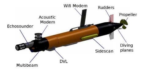
Figure 2.11: The Noptilus Autonomous Underwater Vehicle (AUV)
