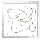
Fig. 9. Robot trajectory while driven manually with constant desired steering angle
