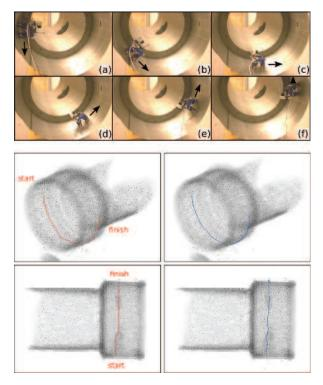
**Fig. 31.** Experiment 1(a): Tracking a circumferential path (using a Hokuyo UTM-30LX point cloud containing 15,000 points). An image sequence of the experiment, followed by plots of the trajectories below. The planned target path is shown on the left, and the actual path as executed by the robot is plotted on the right.
