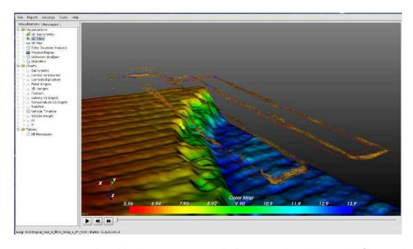
Figure 2.12: Terrain-based localization using a multi-beam sounder and a particle filter on the Noptilus AUV. The bronze cloud around the trajectory is the accumulated particle position over the whole trajectory. The 3D elevation map was realized by processing multibeam echosounder data acquired on a survey mission.
