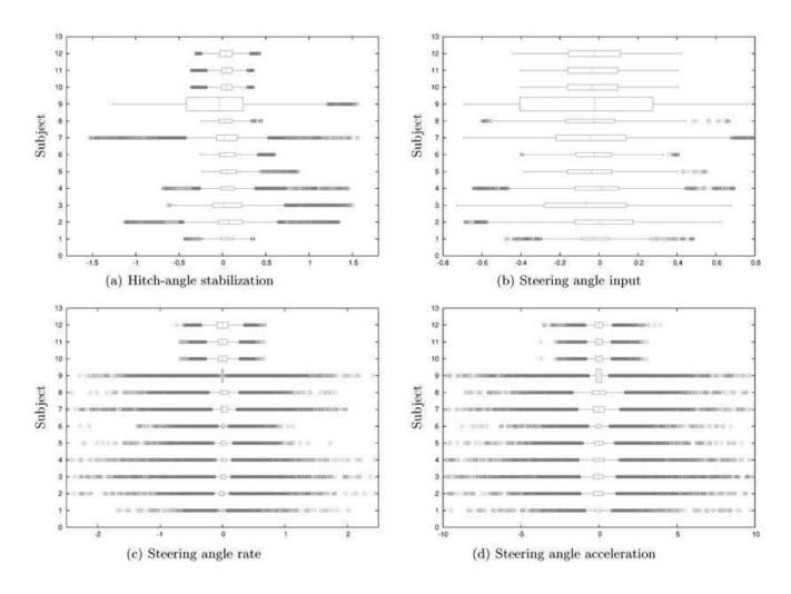
**Figure 16.** Comparisons of the capabilities of human drivers and the autonomous system. Numbers correspond to those given in the Graph label column of Table III. Lines 10–12 correspond to the three runs of the autonomous system.
