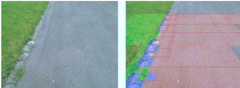
Figure 10. Original image taken from the CRAB (left) and its terrain cell decomposition and prediction using two resolutions (right). The overlay corresponds to the additional predicted cost attributed.
