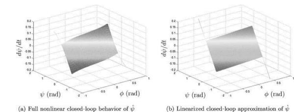
**Figure 6.** Comparison of full and linearized  $\dot{\psi}$  dynamics. Color scale highlights the value of  $\dot{\psi}$ .
