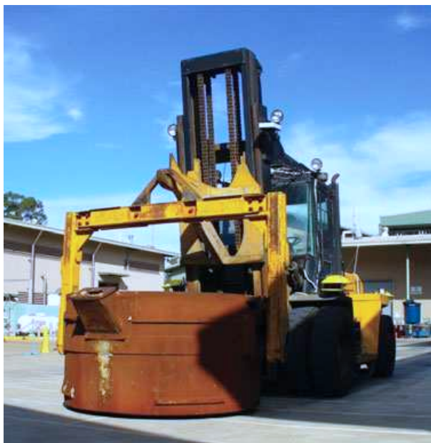
Figure 1. HMC in the process of picking up the crucible.
