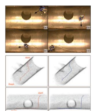
**Fig. 33.** Experiment 2: Avoiding a hole obstacle (using a Hokuyo UTM-30LX point cloud containing 40,000 points). An image sequence of the experiment, followed by plots of the trajectories below. The planned target path is shown on the left, and the actual path as executed by the robot is plotted on the right.
