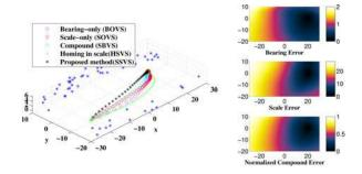
Fig. 4. (Left) Simulated trajectories by different visual homing methods. (Right) Error evaluation on the simulated environment referring to (20,0).
