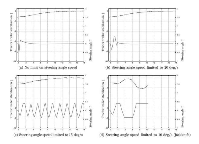
**Figure 7.** Stabilization of a tractor trailer to a straight trajectory using our approach while varying the steering angle speed (simulation). In each graph, the top part of the plot is the path of the vehicle moving from left to right, arrows showing the heading of the tractor and trailer, and the bottom part shows the steering angle during the maneuver.
