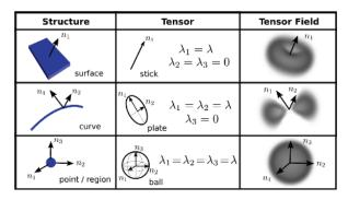
**Fig. 5.** Visualization of tensor voting in three dimensions. The fundamental types of structures are shown in the left-most column. The second column shows the form of the representative 3D tensors, with their eigenvalues  $\lambda_i$ . The last column shows the form of the voting fields cast by each fundamental structure. The vectors representing the structures' normal spaces are illustrated in each column as well. (Adapted from Medioni and Mordohai (2004).)
