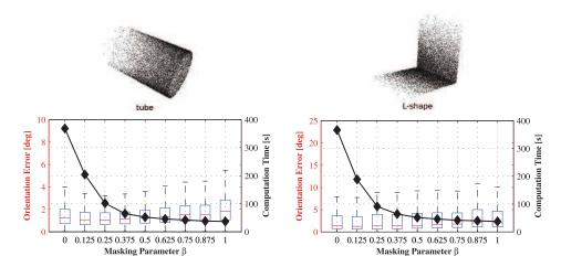
Fig. 20. Error in estimated orientations, predicted from tensor voting performed on a tube structure (left) and an L-shaped structure (right), as well as computation time, as the masking parameter  $\beta$  is varied. Both point clouds contain 24,000 points.
