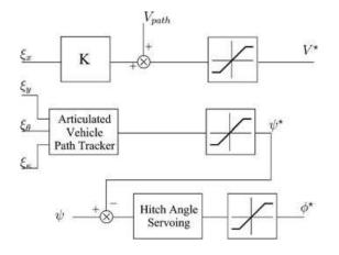
Figure 4. Block diagram for the reversing control law.
