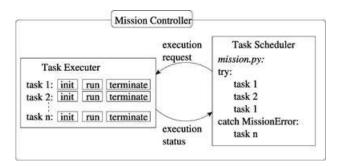
**Figure 9.** Overview of the mission control architecture.
