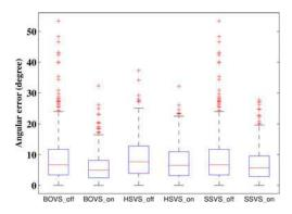
Fig. 13. Error comparison in the cases with/without outlier rejection. The labels marked with \_on indicate the boxplot with outlier rejection and \_off indicates the results calculated from the raw matching result.
