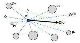
Fig. 1. Abstracted problem of homing. Key points  $p_1$  to  $p_n$  can be observed at the current position C and at the *Home* position O. The variant sizes indicate the differences of key points in scale.
