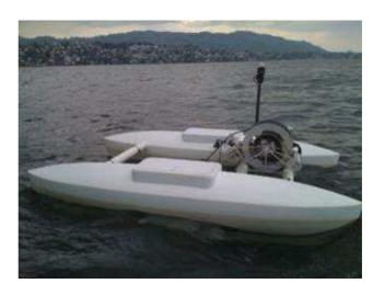
Figure 2.15: Autonomous boat designed at the Autonomous Systems Lab: Avalon (left) and Lizhbeth (right) used in the Limnobotics project (www.limnobotics.ch).
