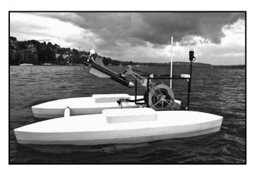
Fig. 1. The autonomous sampling vessel, which is a catamaran 2.5 m long and 1.8 m wide called *Lizhbeth*, during a sampling mission on Lake Zurich. The winch system is used to lower a light sensor and a multi-parameter probe, which is inserted in the plane-shaped fiberglass casing. The casing has elongated perforations to allow the water to reach the sensors. The front tip of the casing is a 4.2 kg steel weight.
