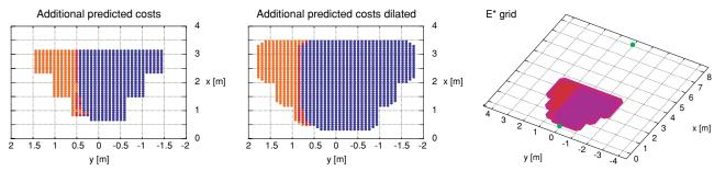
**Figure 9.** Different steps of the terrain prediction. Original prediction (left), dilated prediction (middle), and the resulting E\* grid (right). Note that on the latter, the starting position and goal are depicted with the lighter dots.
