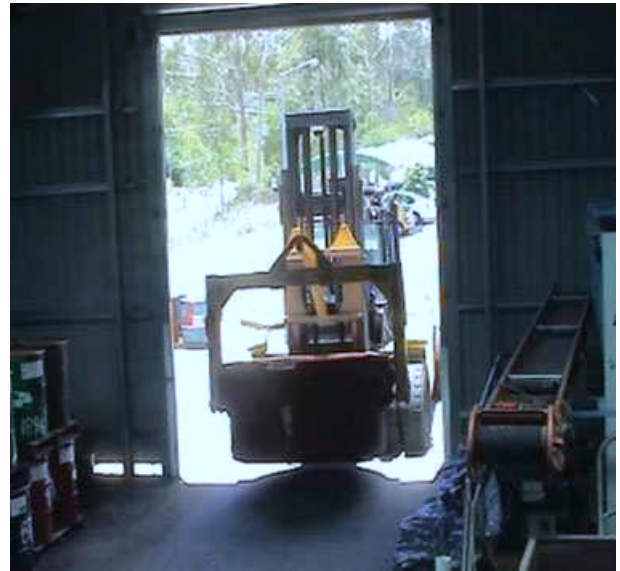
Figure 18. The doorway into the storage shed was narrow for the HMC to enter. There was approximately 30-cm clearance on either side.
