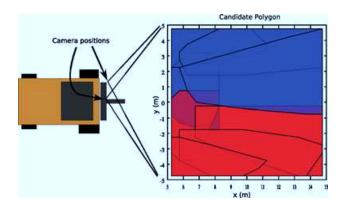
**Figure 16.** Projection of image frames corresponding to selected viewpoint onto the target plane: optimal viewpoint for two cameras while trying to balance the camera use, blue polygons correspond to the area viewed by camera 1; red ones are viewed by camera 2.
