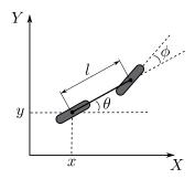
Fig. 17. Simplified front-wheel-drive model of the MagneBike robot.
