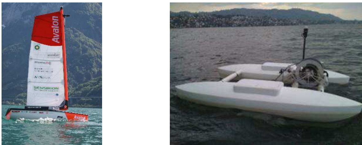
Figure 2.15: Autonomous boat designed at the Autonomous Systems Lab: Avalon (left) and Lizbeth (right) used in the Limnobotics project ( www.limnobotics.ch ).
