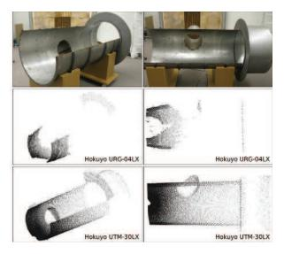
**Fig. 30.** Comparison of two Hokuyo laser range finders, URG-04LX and UTM-30LX, using scans of the test environment. The scans were taken from the bottom of the left end of the tube, with the lasers rotating around a vertical axis. The UTM-30LX shows large improvements in both range and accuracy for this metallic surface.
