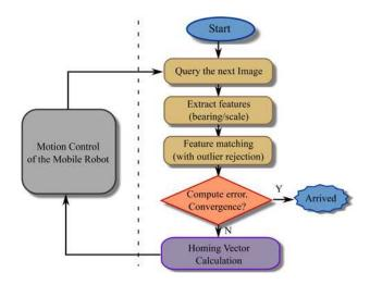
Fig. 2. Control loop of multipoint homing.
