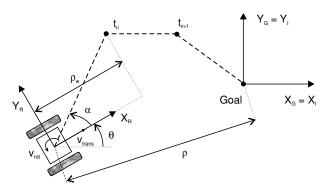
**Figure 6.** Path following for a differential-drive robot.
