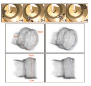
**Fig. 32.** Experiment 1(b): Tracking a circumferential path (using a Hokuyo URG-04LX point cloud containing 22,000 points). An image sequence of the experiment, followed by plots of the trajectories below. The planned target path is shown on the left, and the actual path as executed by the robot is plotted on the right. Note the strong deformations when compared with the point clouds of Figure 31.
