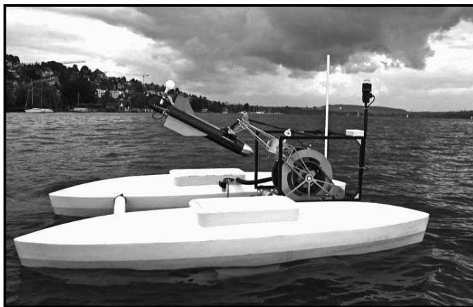
Fig. 1. The autonomous sampling vessel, which is a catamaran 2.5 m long and 1.8 m wide called Lizhbeth , during a sampling mission on Lake Zurich. The winch system is used to lower a light sensor and a multi-parameter probe, which is inserted in the plane-shaped fiberglass casing. The casing has elongated perforations to allow the water to reach the sensors. The front tip of the casing is a 4.2 kg steel weight.
