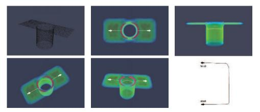
**Fig. 24.** The above results exemplify the ability of the algorithm to provide paths on a highly complex surface. The input point cloud and 2D path are also shown. Here the robot must travel down and around in the tube section in order to cross to the other side of the plate. Note that the edges, which are highlighted, are crossed perpendicularly when entering and exiting the tube section, according to the initially specified requirements on attack angles for step climbing.
