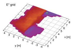
**Figure 21.** Final prediction map of test 4 showing the value of  $\Lambda$  for each one of the observed  $c_l$ . The grass terrain is well recognized and predicted. It corresponds to the area on the left-hand side.
