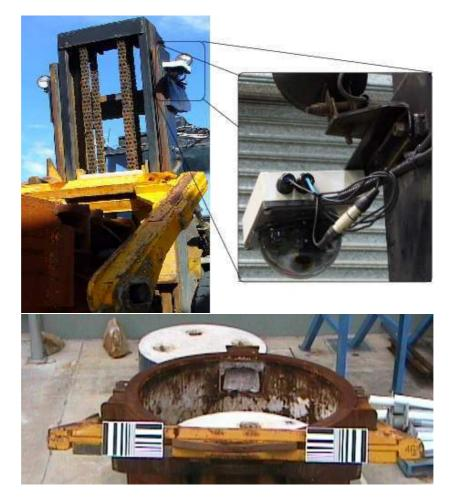
Figure 2.8: Vision setup on the hot-metal carrier. Top camera placement on top of the HMC mast, bottom camera view.
