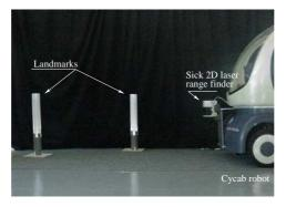
Fig. 2. Cycab robot and its landmarks for localization
