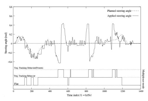
Fig. 18. Applied steering with respect to planned steering, and multiplexer mode.
