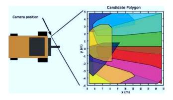
**Figure 14.** Projection of image frames corresponding to selected viewpoint onto the target plane: each polygon shows which part of the target plane is visible with enough resolution in a given frame.
