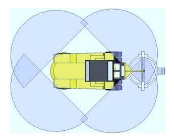
**Figure 3.** The HMC's lasers are located at each corner of the vehicle, tilted down by approximately 4 deg. They offer overlapping coverage out to approximately 30 m. They are used for localization in the navigation phases and for obstacle avoidance.
