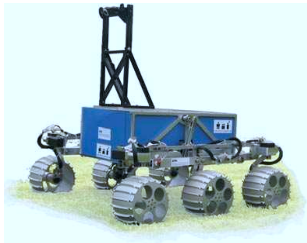
Figure 1. CRAB rover used in the context of this research.
