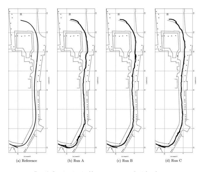
**Figure 14.** Reversing trajectories of the autonomous system on three independent runs.
