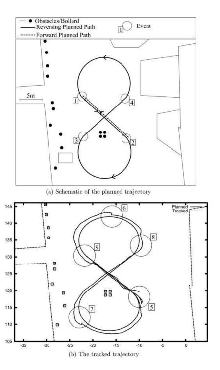
Figure 13. Performance for a poorly planned trajectory that does not account for curvature limitations or path discontinuities. Events are denoted by the boxed numbers.
