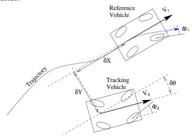
Fig. 11. Variables involved in trajectory tracking behaviour
