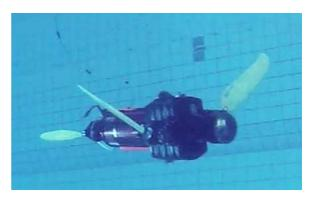
Figure 2.14: Bio-inspired mechatronic design projects: a membrane-based underwater locomotion system inspire by a cuttlefish (left) and underwater system with a kinematic comparable with a sea-turtle (right).
