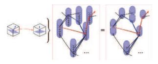
**Fig. 12.** Single nodes from each set of nodes are connected in a sparse graph, due to given constraints in the robot's and surface's orientations, which determine connectivity. According to these constraints, paths may go through the same physical 3D location (i.e. the same set of nodes) but with a different heading, and thus remain unconnected (i.e. different nodes).
