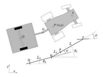
**Figure 1.** Kinematic model of a tractor-trailer system. It is particularly important to note the definition of the steering angle  $\phi$  and the hitch angle  $\psi$ , i.e., the angle between the tractor and the trailer.
