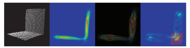
Fig. 9. Extraction of environmental feature maps: surface and edge maps are extracted from the tensor voting results for modeling the environment. The input tokens are shown in the first image, followed by a cross section of the surface saliency map, then a cross section of the surface normal map (scaled by saliency) and finally a cross section of the edge saliency with an overlay of the binary edge map.
