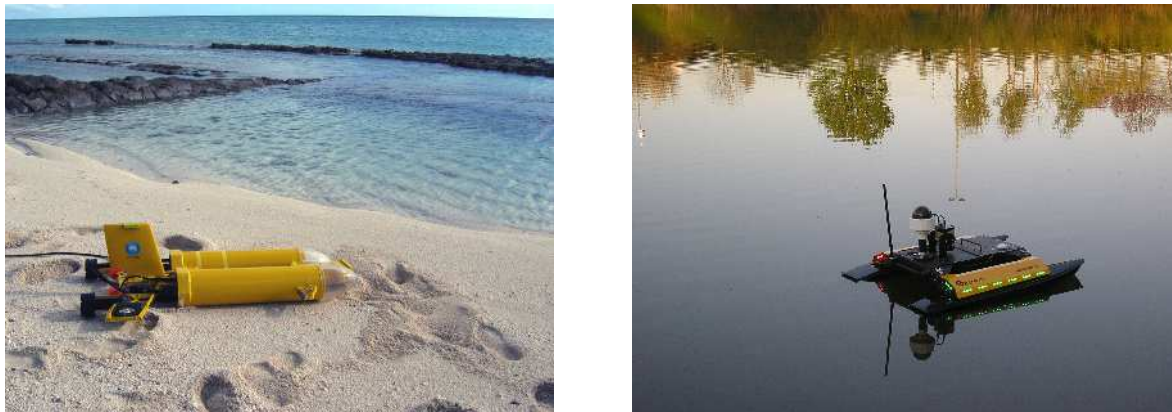
Figure 2.16: Autonomous vehicle specifically designed for environment monitoring: the Starbug AUV from CSIRO (left) and the Kingfisher ASV used at GeorgiaTech Lorraine (right).
