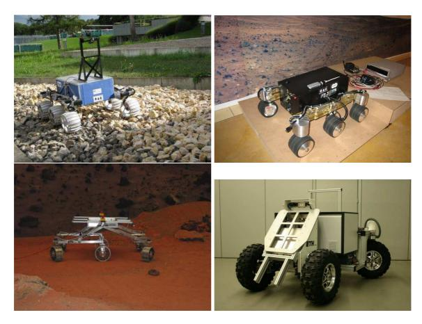
Figure 2.5: Planetary rover prototypes developed at the Autonomous Systems Lab
