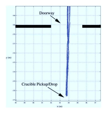
**Figure 21.** The 28 traverses into and out of the storage shed during the 2-h experiment. These paths are contained in an envelope whose radius is less than 15 cm.
