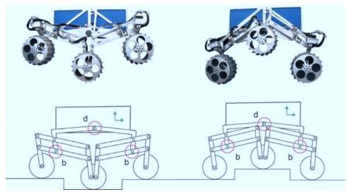
**Figure 5.** CRAB suspension mechanism movement. The position of the angular sensors is depicted with the dashed circles. The four  $MR_b$  (two on each side) are indicated with a b, and the two  $MR_d$  (one on each side) are marked with a d.
