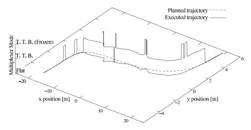
Fig. 16. Executed trajectory with respect to planned trajectory, and multiplexer mode.
