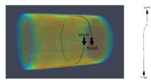
**Fig. 23.** An example of an almost circular path, along with the corresponding unwrapped 2D path. The robot is traveling in a loop on the inside of the tube.
