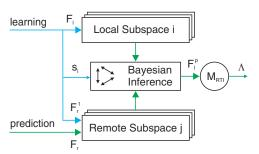
**Figure 8.** Schematic representing the learning and prediction mechanism in the representation chosen for this work (using subspaces). The metric  $\Lambda$  is the function that drives how the path is planned and can be related to the rover's behavior as expressed in Section 2.1.
