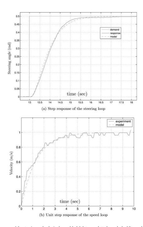
**Figure 9.** Step response of the steering and velocity loops. Model data are plotted as a dashed line and experimental data as a solid line.
