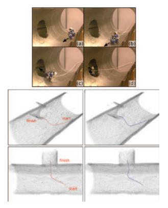
Fig. 34. Experiment 3: Traversing an edge obstacle (using a Hokuyo UTM-30LX point cloud containing 20,000 points). An image sequence of the experiment, followed by plots of the trajectories below. The planned target path is shown on the left, and the actual path as executed by the robot is plotted on the right.
