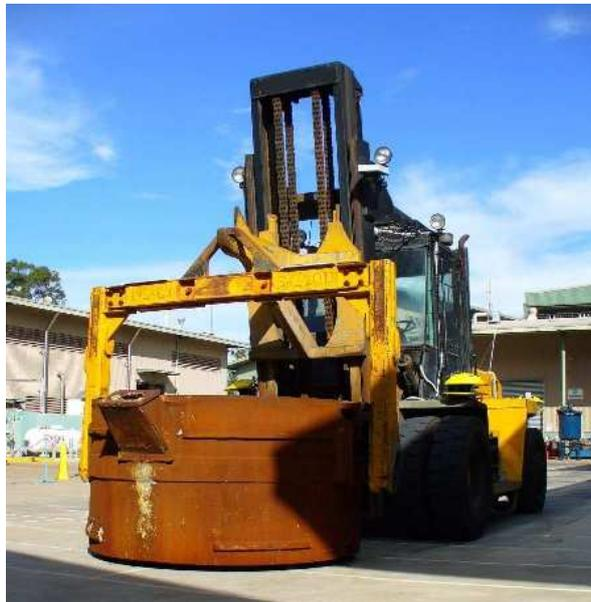
Figure 2.2: The Hot Metal Carrier, a modified forklift for the transport of liquid aluminium
