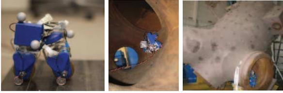
**Fig. 1.** The MagneBike robot and its expected environment. Left: Close-up of the MagneBike robot. Middle: MagneBike inside a steam chest at a junction facing a hole-like obstacle. Right: Outside view of the steam chest, with MagneBike climbing along the tube perimeter.
