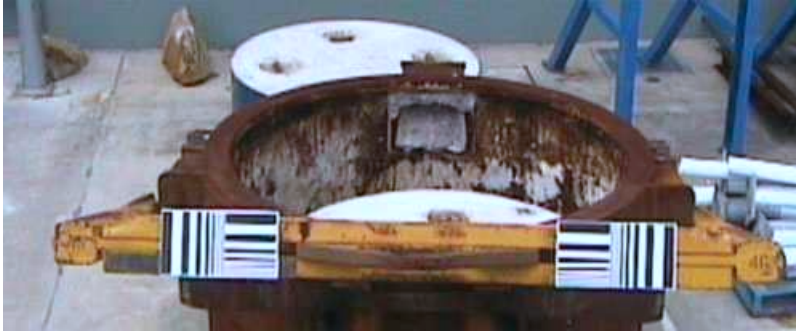
Figure 12. Fiducials and their placement on the crucible (as seen from the PTZ camera).
