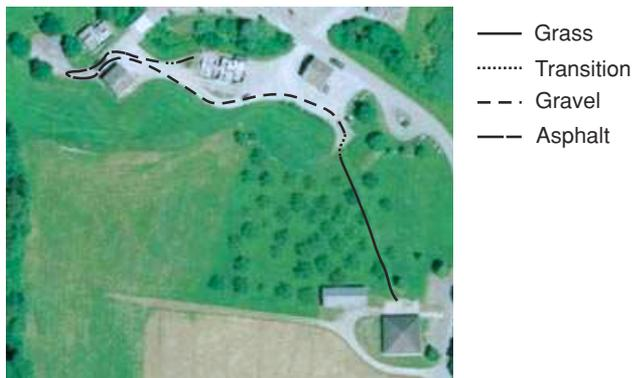
**Figure 15.** Trajectory of the CRAB rover during test 2. Different types of terrains as well as the transition in between can be observed. The terrain classes leave a lot of room for interpretation, because the ground truth is difficult to define.
