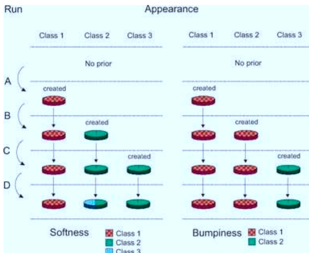
Figure 13. Progress of the rover knowledge during the first test sequence, ABCD. The softness (left) and bumpiness (right) subspaces can be seen in parallel or independently. Their number of elements is alike as it depends on the appearance classes.
