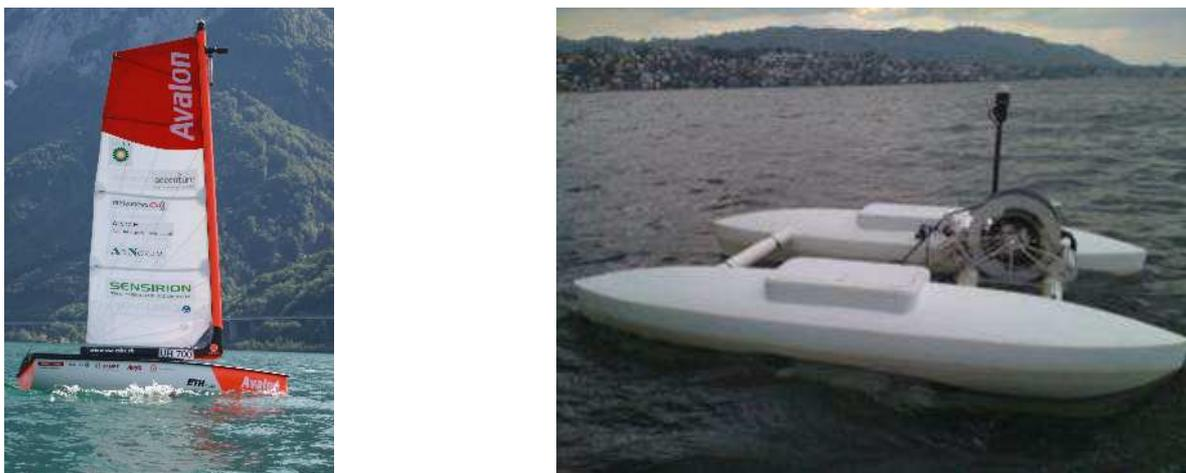
Figure 2.15: Autonomous boat designed at the Autonomous Systems Lab: Avalon (left) and Lizbeth (right) used in the Limnobotics project ([www.limnobotics.ch](http://www.limnobotics.ch)).
