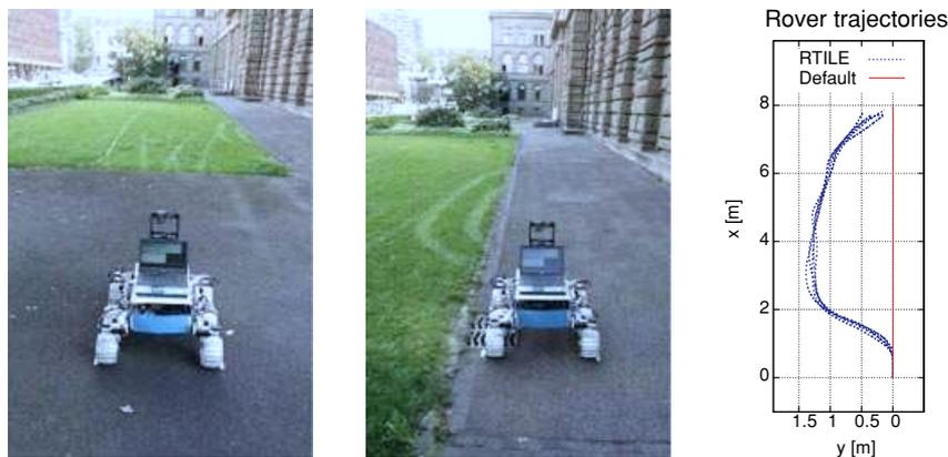
**Figure 20.** Test 4: CRAB rover at the starting point of first part (learning phase on the left-hand side), of the second part (middle), and resulting test trajectories (right). The traces left by the rover in the grass during the previous trial can be observed.
