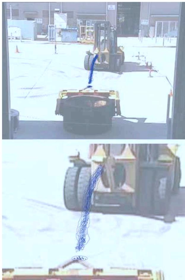
**Figure 20.** Pickup approach trajectories: superimposition of 29 pickups. The dots and the ellipse around the crucible handle show the variability of the crucible location across this set of maneuvers. The top figure shows an overview of the experiment area, and the bottom figure shows a close-up on the paths themselves. For reference, the handle width is about 2 m and the pickup hole approximately 20 cm across.
