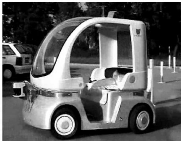
Figure 2.1: The CyCab: an autonomous car-like vehicle for urban mobility
