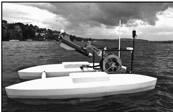
Fig. 1. The autonomous sampling vessel, which is a catamaran 2.5 m long and 1.8 m wide called Lizbeth , during a sampling mission on Lake Zurich. The winch system is used to lower a light sensor and a multi-parameter probe, which is inserted in the plane-shaped fiberglass casing. The casing has elongated perforations to allow the water to reach the sensors. The front tip of the casing is a 4.2 kg steel weight.
