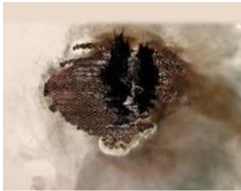
Figure I.11. Damage of carbon fibers tows at the lightning attachment point (Source: National Institute for Aviation Research (NIAR))
