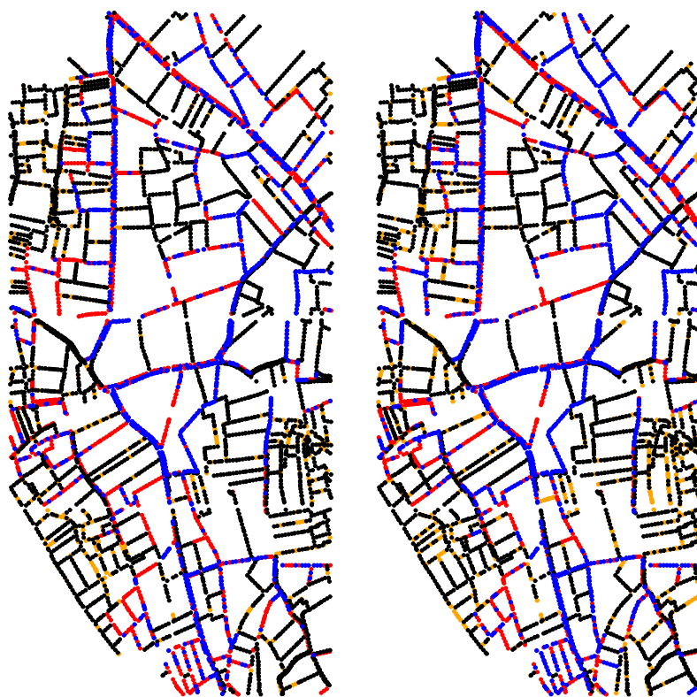
FIG. 4.9 – Maps of classification results using wavelets (right) or watershed (left) on study area : blue points are for D well classified sites, red for ditches omission, orange for ditches commission and black for ND well classified sites
