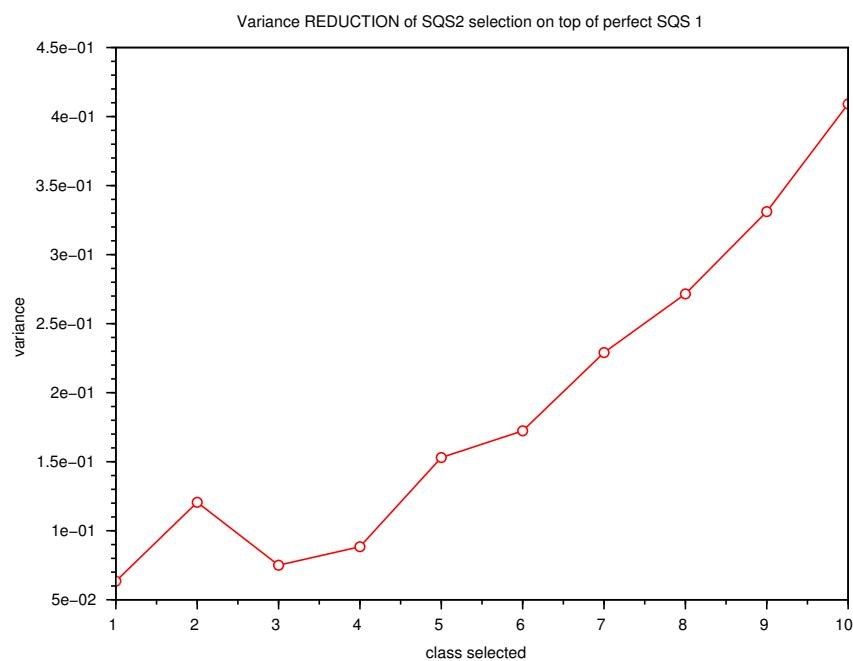
Figure 4.4 – Variance ratio  $\frac{V_{\text{SQS 2}}}{V_{\text{exact SQS 1}}}$  for the different groups of realizations (sorted according to their SQS 2 error; the SQS 1 condition is exactly satisfied). Only the 10 best groups are shown.
