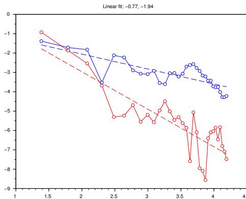
Figure 3.11 – Errors (3.62) as a function of  $N$  ( $M = 100$ ; log-log plot). Blue curve (with slope -0.77): Monte-Carlo approach. Red curve (with slope -1.94): Control Variate approach using (3.39). The reference value has been computed using  $N_{\text{ref}} = 100$  and  $M_{\text{ref}} = 100$ .
