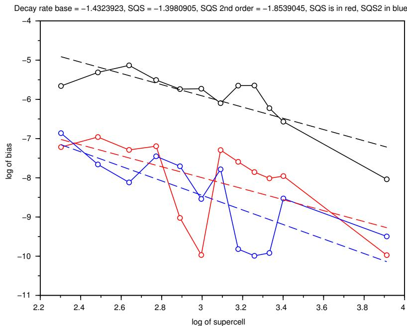
Figure 4.8 – log-log plot of the total error as a function of the supercell side length  $N$  (natural logarithm). Black curve: Monte Carlo method. Red curve: SQS 1 method. Blue curve: SQS 2 method (see text).
