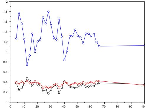
Figure 3.10 – Optimal values of  $\rho_1$  (black),  $\rho_2$  (red) and  $\rho_3$  (blue) for the controlled variable (3.39) as a function of  $N$ . We have considered all values  $N \in \{4, 6, \dots, 66\}$  as well as  $N = 100$ .
