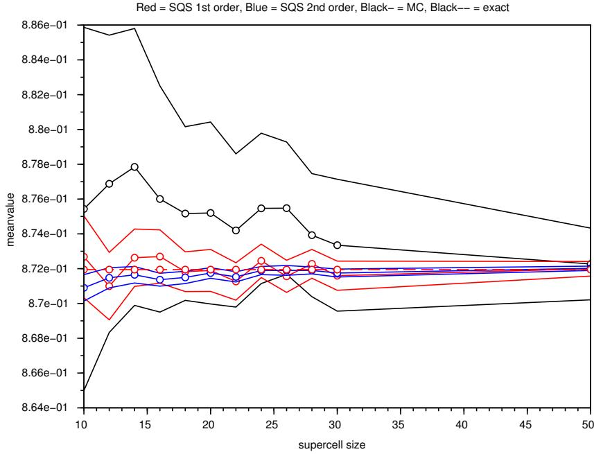
Figure 4.7 – Estimators of  $[A^*]_{11}$  (along with confidence intervals) as a function of the supercell side length  $N$ . Black curve: Monte Carlo method. Red curve: SQS 1 method. Blue curve: SQS 2 method (see text).
