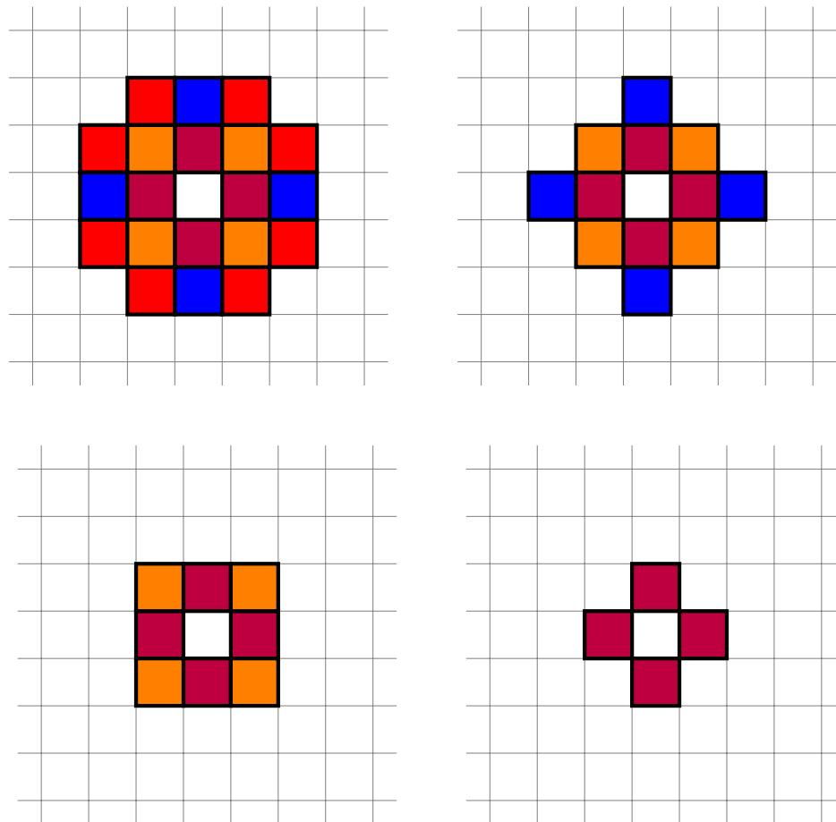
Figure 3.7 – Sets  $\mathcal{N}_N$  of position of second defect that we consider to build the RB basis set (the first defect is always in the central white cell). Top left: Card  $\mathcal{N}_N = 20$ . Top right: Card  $\mathcal{N}_N = 12$ . Bottom left: Card  $\mathcal{N}_N = 8$ . Bottom right: Card  $\mathcal{N}_N = 4$ .
