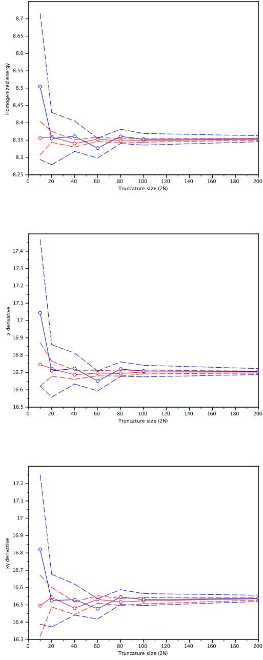
Figure 2.1 – Test-Case 1: Homogenized quantities as a function of  $2N$ , for the vector  $\xi = (1, 1)^T$  (Blue: Monte Carlo results; Red: Antithetic variable approach; Dashed lines: 95% confidence interval, equating the cost of the two approaches). From top to bottom: estimation of  $\mathbb{E}[W_N^*(\cdot, \xi)]$ ,  $\mathbb{E}[\partial_{\xi_1} W_N^*(\cdot, \xi)]$  and  $\mathbb{E}[\partial_{\xi_1 \xi_2}^2 W_N^*(\cdot, \xi)]$ .
