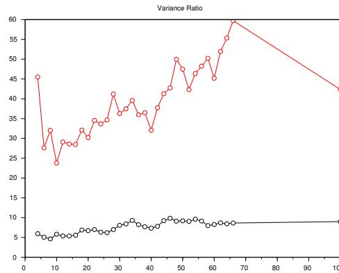
Figure 3.9 – Variance ratio (3.60) as a function of  $N$ . Black curve: using the first order controlled variable (3.31). Red curve: using the second order controlled variable (3.39). We have considered all values  $N \in \{4, 6, \dots, 66\}$  as well as  $N = 100$ .
