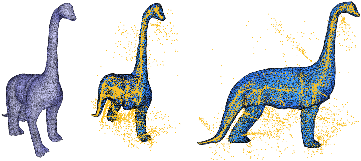
Figure 4.7: The “Dino” surface (leftmost). An isotropic mesh of the “Dino” surface (middle and rightmost) and its poles (yellow).
