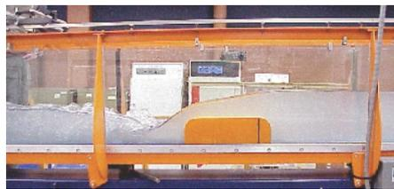
Figure 5.5: Hydraulic jump experiment
