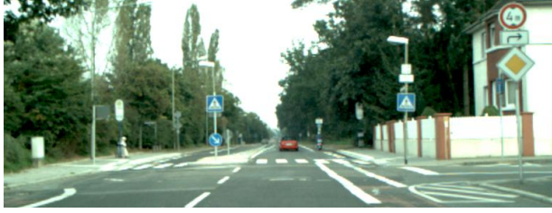
Figure 2: Traffic sign detection as an example of object detection with diagnostic features. In this case, the feature in question is color, as the blue, yellow or red colors of the shown traffic signs give already a very good indication about their presence and position.
