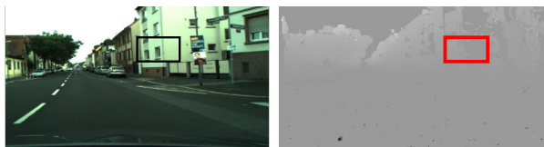
Figure 26: Examples of stereo processing for elevation and distance calculation in the context-based object detection architecture. a) video image b) dense elevation map (brighter pixels are higher over the ground plane).
