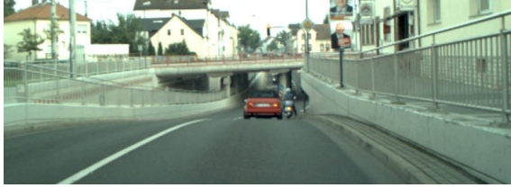
Figure 3: Uncontrolled environments prevent simple hypotheses: in the shown traffic situation, the usual assumption of a flat ground plane is no longer valid. If the ground plane hypothesis is used to give a priori indications about object positions, its application would even be harmful here, as the system would suddenly detect many objects that have no link at all with the true (curved) ground plane.
