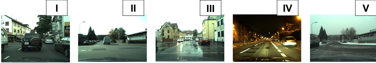
Figure 4: Examples of the effect that time of day and weather can have on a visual image, the starting point for visual perception. The ideal climatic condition, an overcast sky without direct sunlight, is shown in I. In II, it can be observed what direct, low-standing sun can do in the way of shadows which are very detrimental to detection algorithms. In III, we observe that rain completely changes the appearance of a visual scene, with a reflective road surface that may even lead to "ghost detections", i.e., the detection of vehicles that are reflected on a wet road. In IV, the effect of night-time is illustrated. Contrary to intuition, the effect is not really dramatic as artificial illumination is usually homogeneous and diffuse and thus does not cause strong shadows. In V, the effects of fallen snow can be inspected. This case does not present extreme challenges to visual processing, but LIDAR signals are strongly affected due to the high reflectance of snow and ice.
