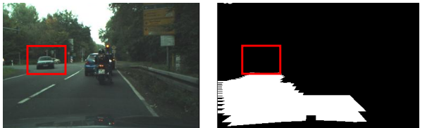
Figure 25: Performance example of free-area computation. a) Video image b) computed free area as a binary mask.
