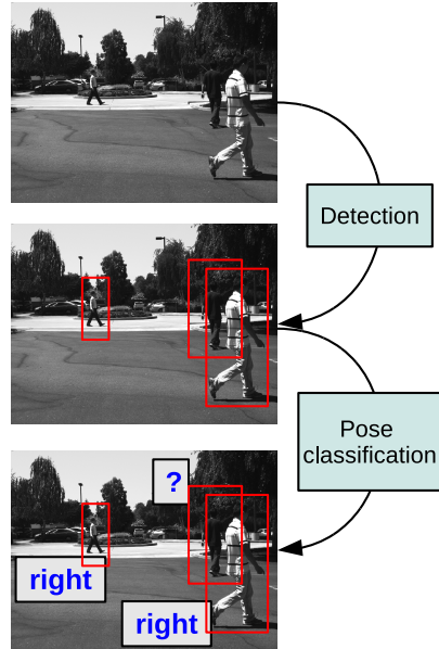
Figure 18: Block diagram of the real-time pedestrian detection/pose classification system, which is composed of a detection and a pose classification stage.
