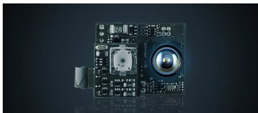
Figure 12: The used time-of-flight 3D sensor for gesture classification, the Camboard Nano. Due to its small dimensions and cheap price, it is well suited for automotive applications.
