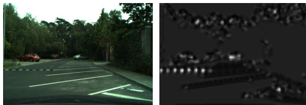
Figure 24: Example of how the appearance-based classifier works in the context-based object detection architecture: for each input image (a) , it produces a retinotopic, dense map of vehicle confidences (b) . This means that each pixel in this map represents the presence or absence of a vehicle, at a specific scale, centered on that pixel.
