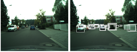
Figure 55: Results of the restricted vehicle detector presented in [73]. Left: original image. Right: vehicle detections. Please note that all vehicles are detected but many incorrect detections exist as well.
