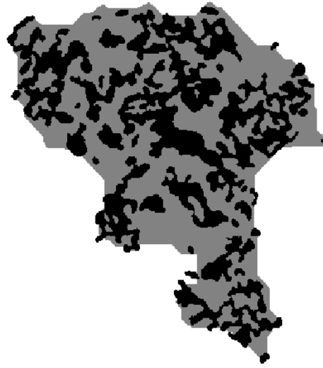
Figure 8.12: Porous volume of the tomography image after closing with rhombicuboctahedron of 30 voxels and erosion by 3 voxels (2D section). Alumina grains are in dark, while in grey is the porosity.
