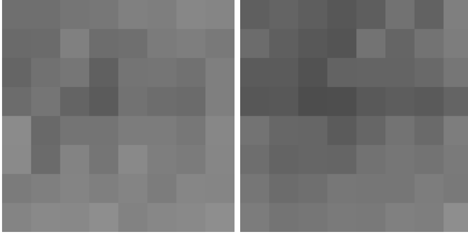
Figure 6.5: Local means computed over a set of non-overlapping square subdomains in two TEM images.
