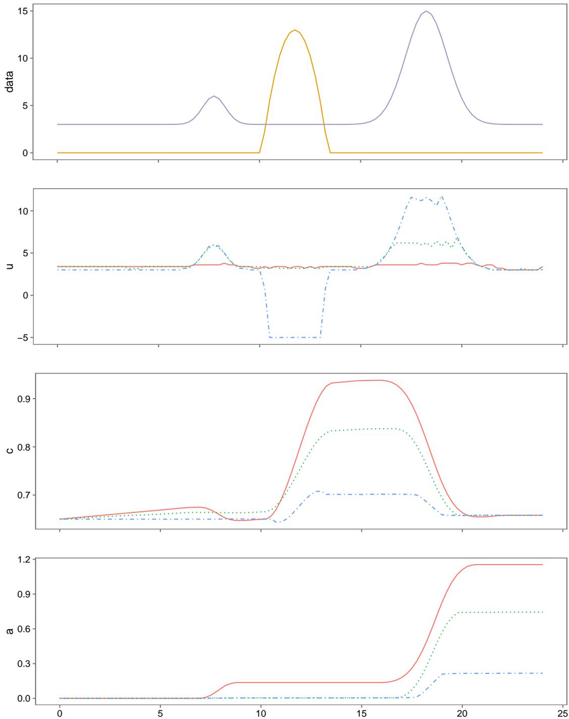
Figure 4.3 – Three simulations for  $(\alpha, a)$  equal to  $(0, 0)$  (solid),  $(0, 400)$  (dot and dash) and  $(250, 0)$  (dot). The bell shaped curve correspond to the solar production  $P_s$  and the other one to the load  $P_L$ .
