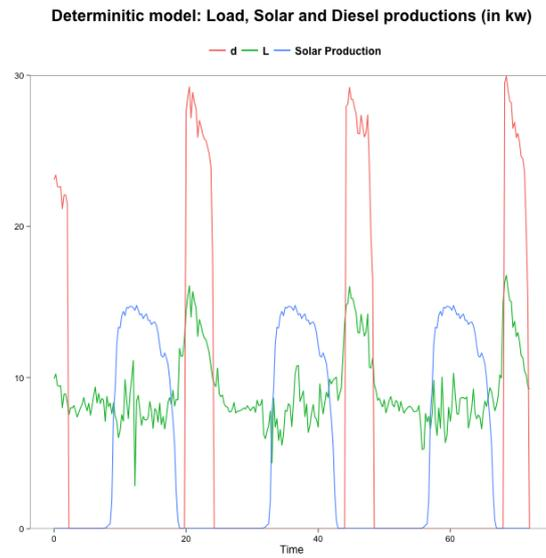
Figure 3.8 – Load and Production for the deterministic simulation (in kW)
