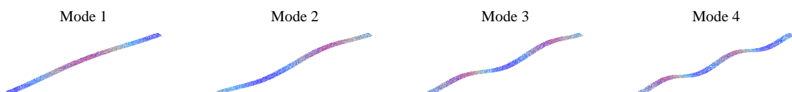
Figure 4.6 - Mode shapes of the nominal model.
