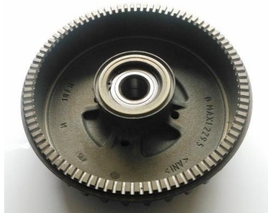
(b) Detection track on the brake drum
