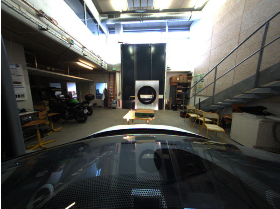
Figure 5.7 – Camera-LIDAR calibration with a circular target example frame
