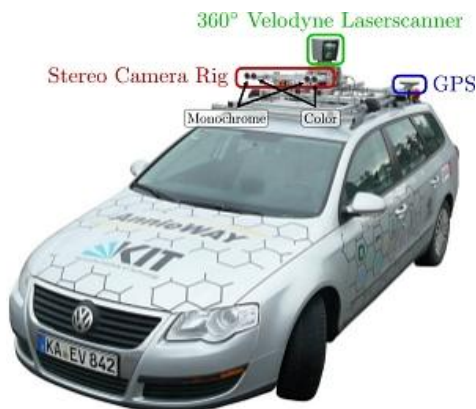
Figure 3.6 – The KITTI dataset used for the experiments is recorded from a moving car equipped with several cameras, a GPS device and a Velodyne LIDAR device.
