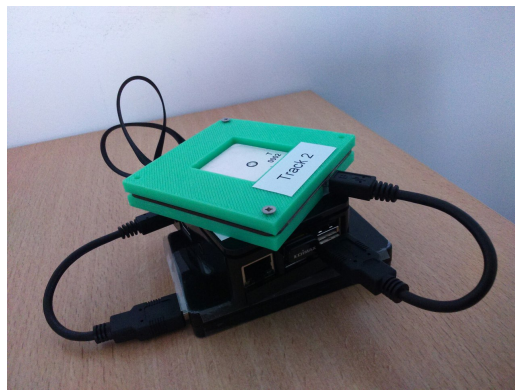
(b) The Raspberry-Pi device with U-blox U8 receiver, battery and WiFi antenna
