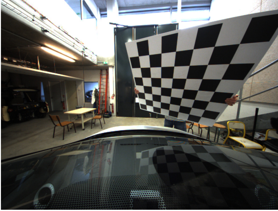
Figure 5.6 – Example frame of checker-board inner camera calibration
