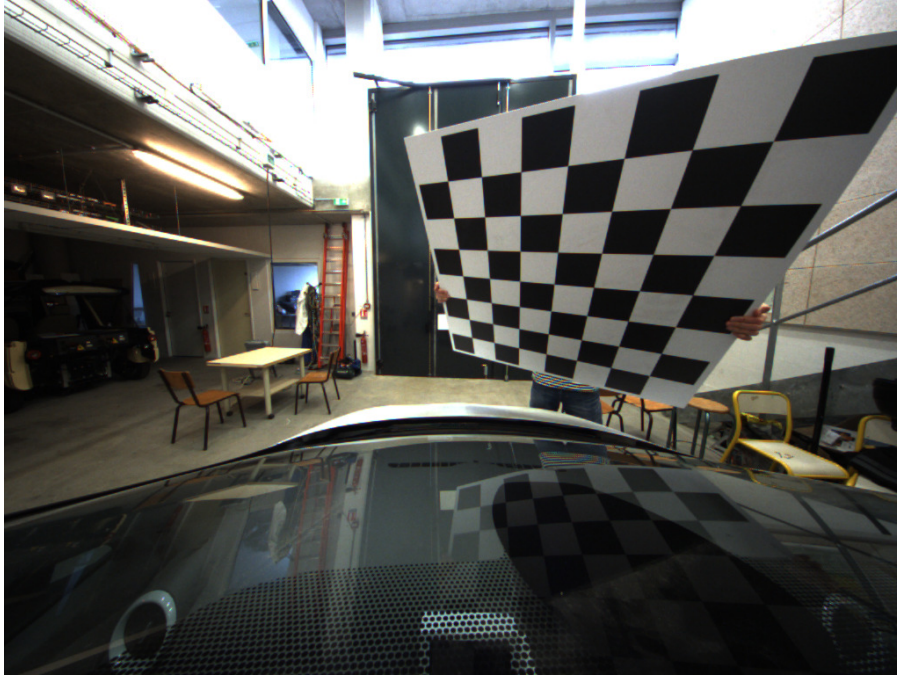
Figure 5.6 – Example frame of checker-board inner camera calibration
