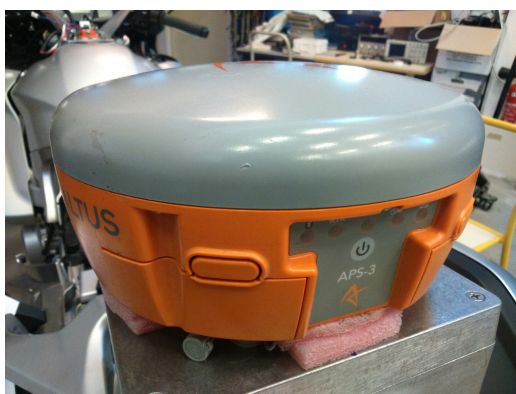
(a) The Altus APS 3 smart antenna
