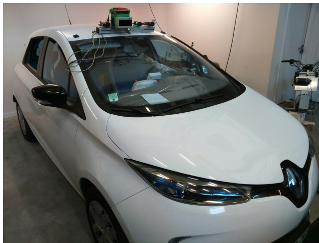
Figure 1 – ZOE - experimental platform of SATIE Laboratory, University Paris Saclay
