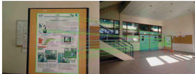
Figure 1.13: The result of visual landmark detection using 2-points RANSAC.
