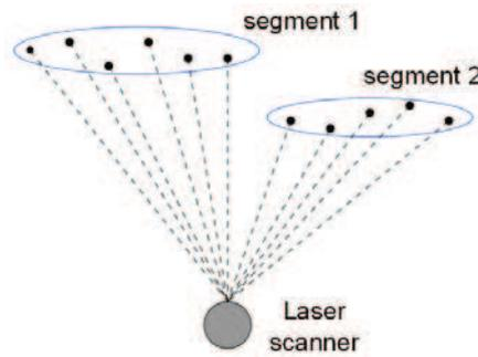
Fig. 2.3: Segmentation using Successive Edge Following algorithm.
