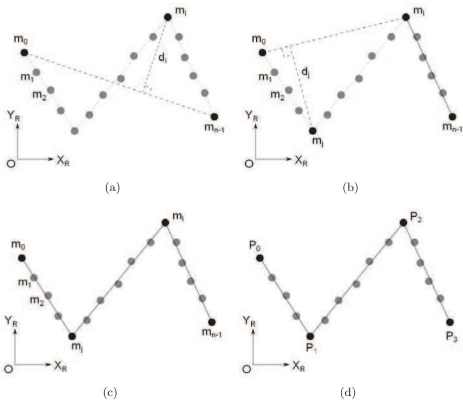
Fig. 2.7: Split-and-merge algorithm applied to a point set.
