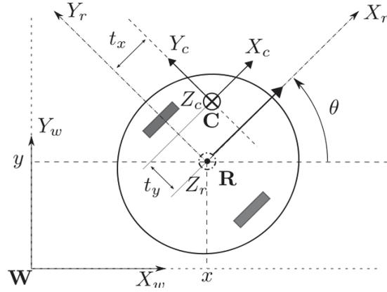
Figure 3.24: Robot-camera configuration using the selected spherical image coordinate.
