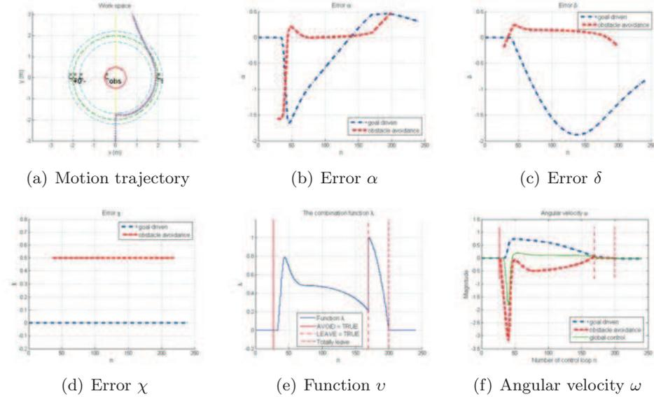
Fig. 2.18: obstacle avoidance simulation using PFM: smooth switching
