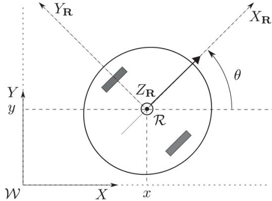
Figure 2.12: Illustration of robot configuration using unicycle model.
