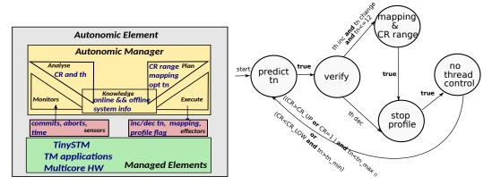
(a) The instantiation of MAPE-K-shape feed- (b) The structure for the autonomic manager of back control loop. Fig.6.2(a) in an automaton shape.
