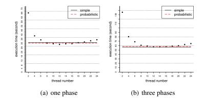
Figure 4.13: Time comparison of static and adaptive parallelisms for **EigenBench** on UMA. The dots represent the execution time with static parallelism.
