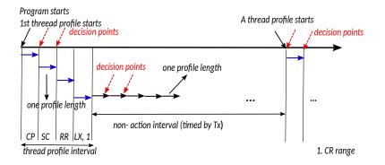
Figure 5.2: Profiling procedure for obtaining the optimum thread mapping strategy.
