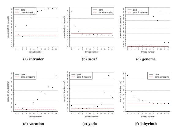
Figure 6.5: Time comparison for **STAMP** for static parallelism, *dynamic parallelism model* and *dynamic thread control model*. The dots represent the execution time with different static parallelism.
