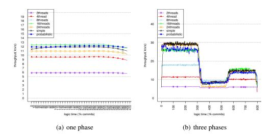
Figure 4.17: Throughput comparison for **EigenBench** on UMA. Fig. 4.17(a) presents the regression curve of the throughput over time, meaning that the throughput has been smoothed. Fig. 4.17(b) illustrates the original data to better present the clear phase change.
