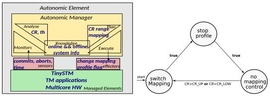
(a) The MAPEK-shape feedback control loop.
