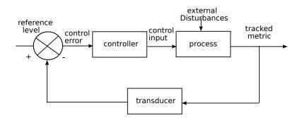
Figure 2.10: The feedback control loop from control theory.
