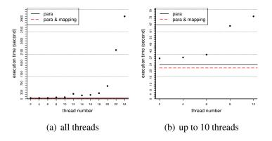
Figure 6.4: Time comparison of **EigenBench** for static parallelism, *dynamic parallelism model* and *dynamic thread control model*. The dots represent the execution time with different static parallelism.
