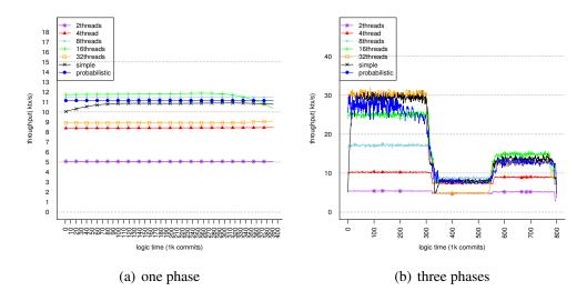
Figure B.1: Throughput comparison for **EigenBench**. Fig. B.1(a) presents the regression curve of the throughput over time, meaning that the throughput has been smoothed. Fig. B.1(b) illustrates the original data to better present the clear phase change.
