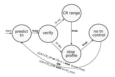
Figure 4.6: The controller of the probabilistic model described as an automaton. th stands for throughput and tn means the thread number.
