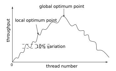
Figure 4.4: Throughput fluctuation. The throughput fluctuates before reaching the maximum point.
