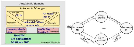
(a) The MAPEK-shape feedback control loop.
