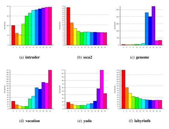
Figure 4.10: Time comparison for **STAMP** for static parallelism on UMA.
