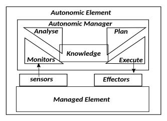
Figure 2.9: A MAPE-K control loop. It incorporates an autonomic manager, a sensor, an effector and a managed element among which the autonomic manager plays the main role.
