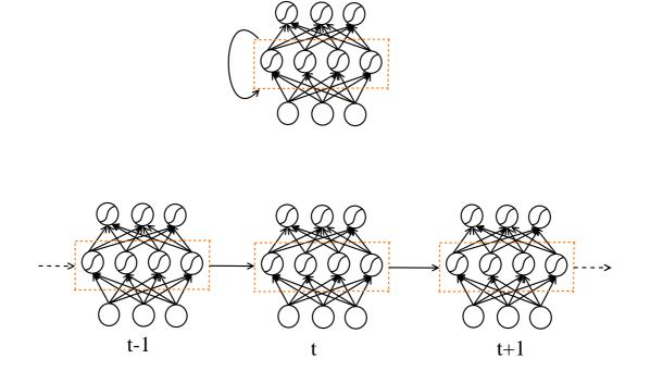
FIGURE 5.9: Architecture of a simple RNN with one hidden layer. Both compact (top) and unfolded in time (bottom) views are presented.
