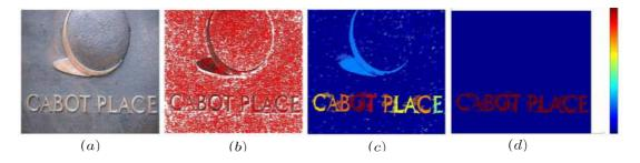
FIGURE 2.5: Text detection method used in [HQT14]. (a) Original image, (b) MSER component candidates, (c) component confidence map after applying ConvNet and (d) final detection after a simple thresholding.
