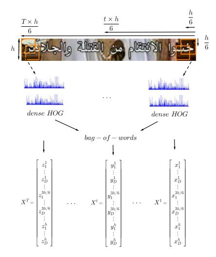
FIGURE 5.17: HOG-based text feature extraction.
