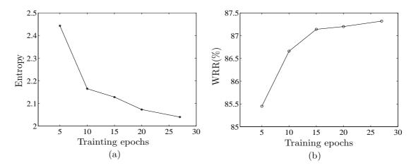
FIGURE 6.5: Evolution of the RNN-700 LM results during training: (a) progressive reduction in the entropy per character on the  $TEXT\_Test$  set. (b) a corresponding improvement in WRR after joint decoding applied to the  $DEV\_Set$  text images, using the RNN-700 configuration after each training epoch.
