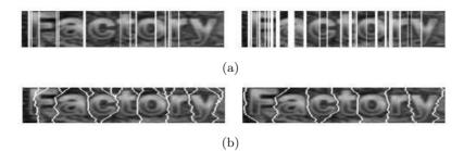
FIGURE 2.9: Character segmentation with both profile projection analysis (a) and the method based on gradient vector flow proposed in [PSST11] (b). (a) illustrates missed segmentation (left) and over-segmentation (right). (b) presents the forward pass (left) and backward pass (right) results of the proposed path finding method.
