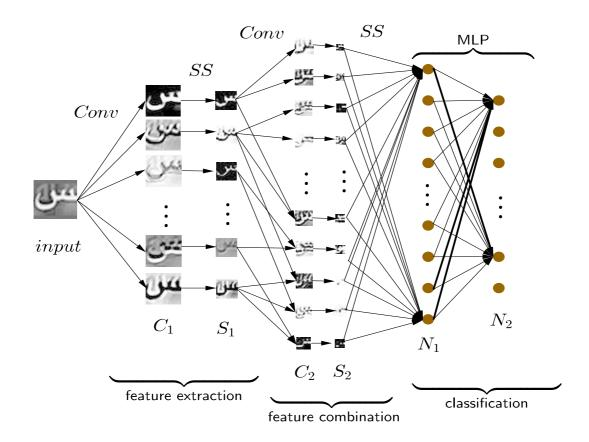
FIGURE 5.7: ConvNet-based character classifier. 'Conv' and 'SS' refer to convolution and sub-sampling operations respectively.
