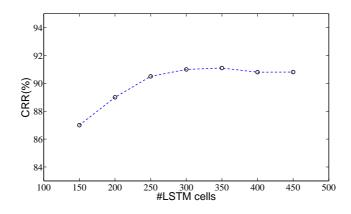
FIGURE 5.16: Impact of the number of LSTM cells.
