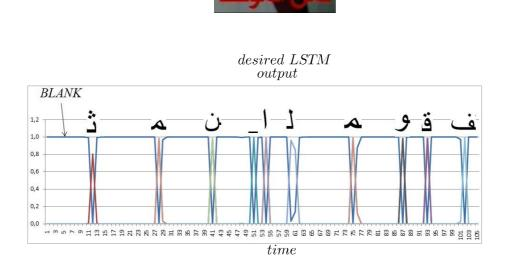
FIGURE 5.12: LSTM/RNN target output units activation through time. Curves represent the activation level through time of a set of label classes (label probability). '\_' corresponds to the space character. Most of times the network emissions correspond to the 'BLANK' class.
