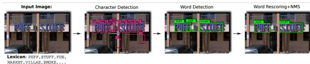
FIGURE 2.12: End-to-end text recognition framework used in [WBB11].
