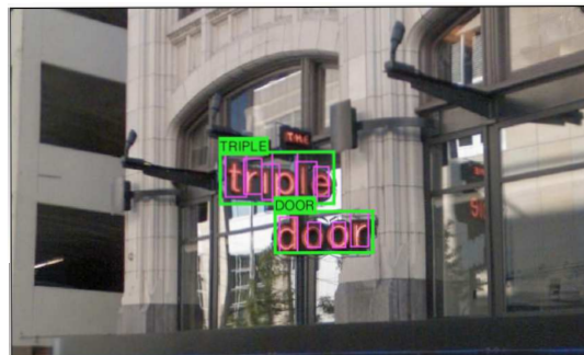
FIGURE 2.3: Text detection and recognition in [WB10]. Characters recognized using HOG features and merged into words using pictorial image.
