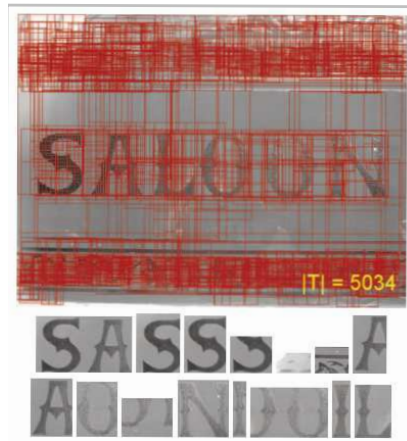
FIGURE 2.2: Examples of character-based candidate regions obtained in [NM13b]. Top image corresponds to bounding boxes of strokes.
