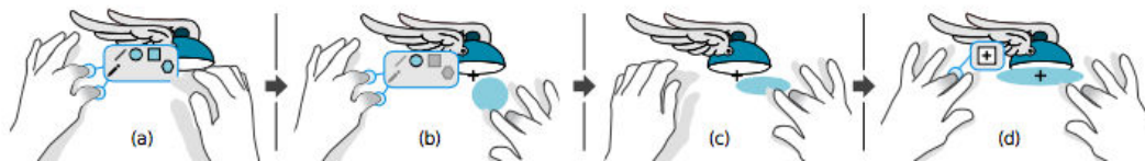
Figure 119: (a) Performing a chording gesture of the NDH determines and displays the corresponding command mapping. In this example, 5 drawing tools are displayed. (b) Using the middle finger to trigger the drawing of an eclipse. (c) The movement of the DH controls the size of the eclipse. (d) Another chording gesture of the NDH adds a constraint for the drawing (Goguey et al., 2014a).
