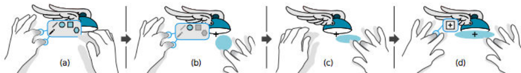
Figure 119: (a) Performing a chording gesture of the NDH determines and displays the corresponding command mapping. In this example, 5 drawing tools are displayed. (b) Using the middle finger to trigger the drawing of an eclipse. (c) The movement of the DH controls the size of the eclipse. (d) Another chording gesture of the NDH adds a constraint for the drawing (Goguet et al., 2014a).
