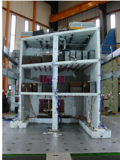
Figure 3.39: Picture of SMART 2013 specimen fixed on the AZALEE shaking table, ready to be tested.
