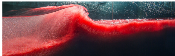
Figure 4.12: Bed mobilization at the breakpoint (photos by Cyril Fresillon - CNRS photothèque).
