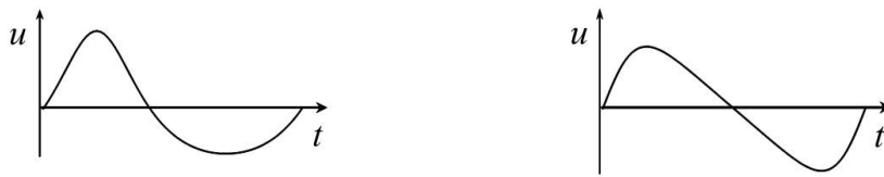
Figure 2.8: Sketch of a velocity-skewed flow (left) and an acceleration-skewed flow (right) (Abreu, 2011).
