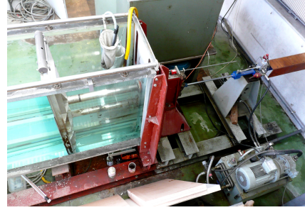
(b) Piston-type wave-maker.
