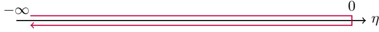
Figure 1.4: Closed time path of the Schwinger-Keldish (in-in) formalism. By defining the field on this time path \mathcal{C} , one can construct the generating functional for expectation values similarly to the generating functional for matrix elements in the in-out formalism.
