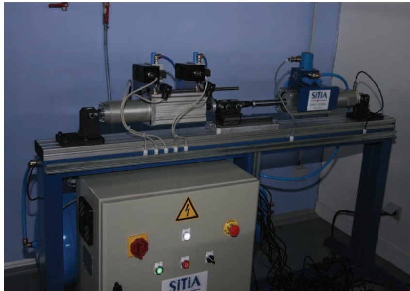
Figure 9.1 – Photo of electropneumatic system
