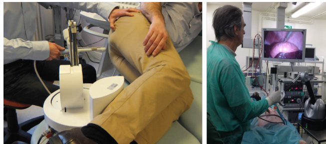
Figure 1. Comanipulating an instrument through a fulcrum: left – the 6 DOFs robot Apollo assists a urologist who manipulates an endorectal ultrasound probe to perform prostate biopsies, [5]; right – the same concept applied to endoscopic surgery
