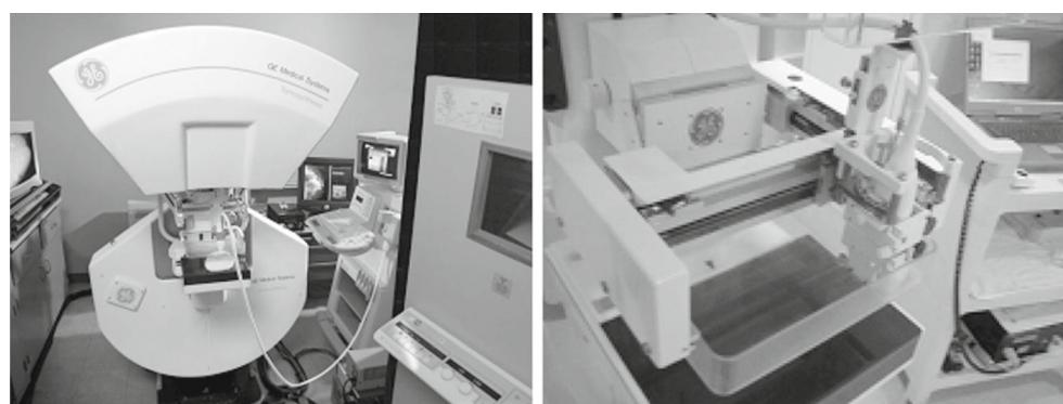
**Fig. 3** Semi-automated US breast scanning system [14]
