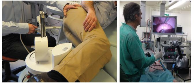
Figure 1. Comanipulating an instrument through a fulcrum: left – the 6 DOFs robot Apollo assists a urologist who manipulates an endorectal ultrasound probe to perform prostate biopsies, [5]; right – the same concept applied to endoscopic surgery
