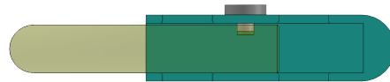
(b) Stereoscopic transmission mechanism composed by a sliding bar and a guiding rectangular tube.
