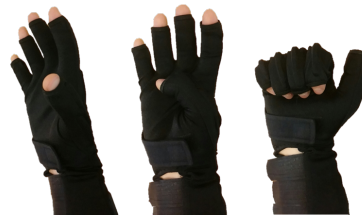
Figure 6.3 – Dataglove calibration postures. From left to right: thumb and finger minimum joint angles, thumb maximum joint angle and finger maximum joint angles.
