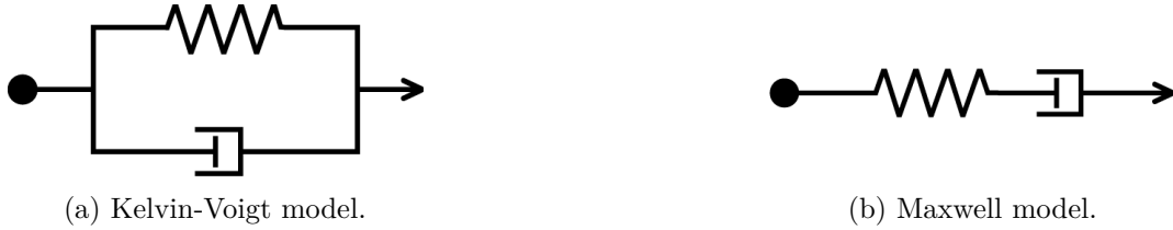
Figure 1.17: The two simplest models of viscoelastic materials, with an elastic response (spring) and a viscous response (damper).
