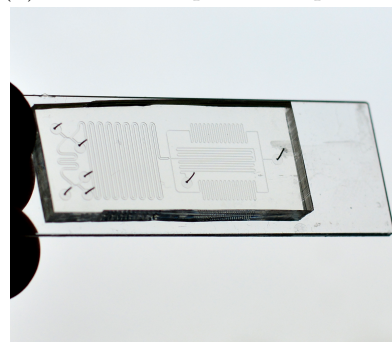
(d) PDMS microfluidic chip: PDMS sealed on PDMS-covered glass.
