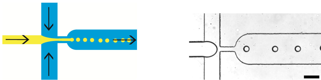
(a) Flow-focusing device: oil (yellow) is pushed with water (blue) through a constriction. The coflow is destabilized into small droplets.
