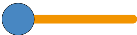
(a) A classic surfactant molecule is composed of a polar head (blue) and a non-polar tail (orange).
