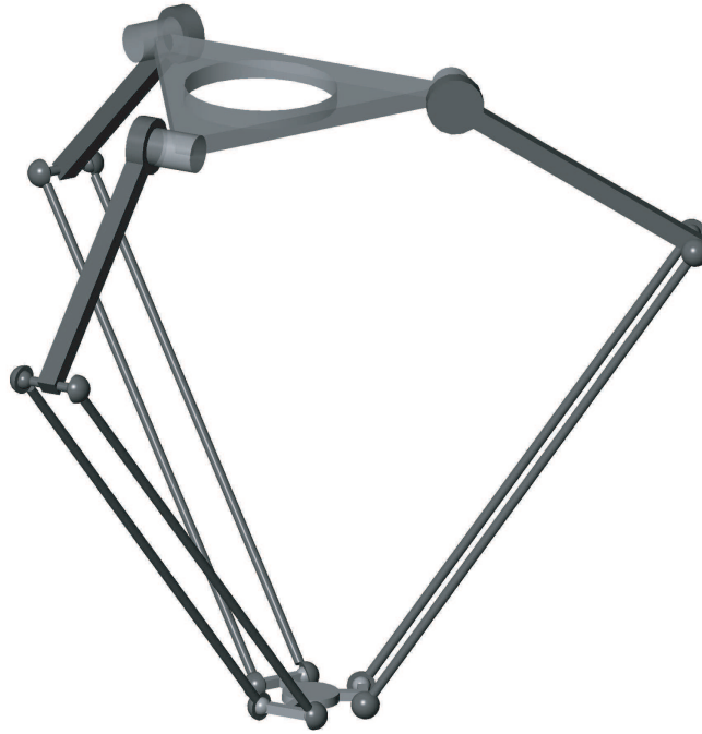
Figure 1.8 – Basic Delta architecture
