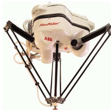
FIG. 2.35 – Le robot Delta
