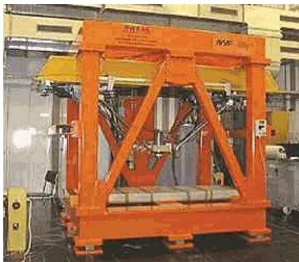
FIG. 2.19 – Machine Hexaglide
