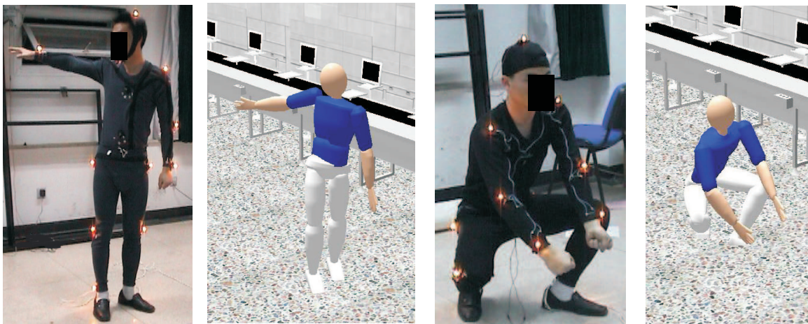
Figure 2.5: Posture comparison between real postures and postures in simulation
