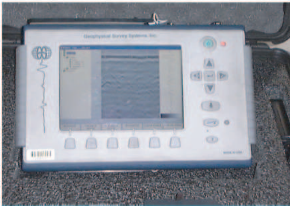
Figure 1.1: Example of an impulse GPR (SIR-3000) [5]
