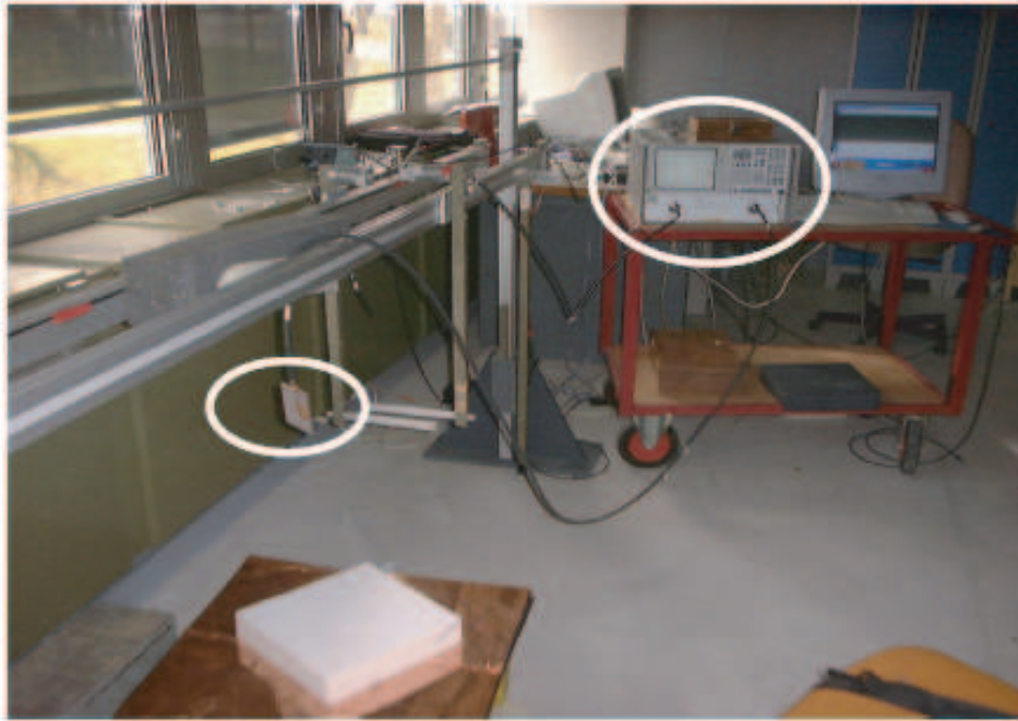
Figure 1.2: Example of a step frequency GPR [5]
