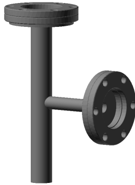
Figure 2.6: Drawing of the oven. The lithium is lying at the bottom of the vertical tube, which is heated up at 500^{\circ}\text{C} .
