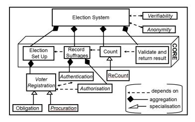
Figure 26: Adding Features To Architecture
