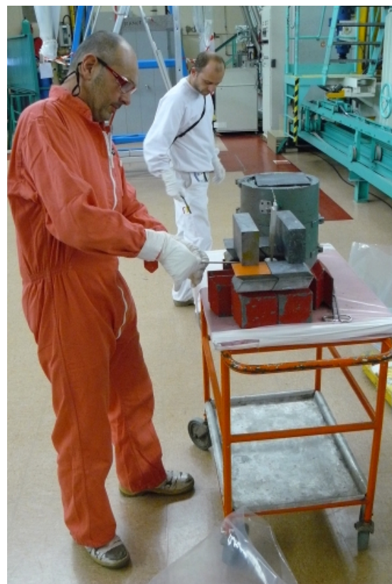
(c) Post irradiation dismantling of shuttle load element. E. Mannino doing the operation under P. Cochet supervision.
