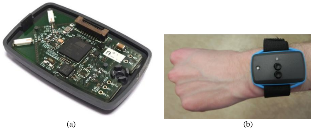
Figure 2.1. (a) Zyggie hardware platform showing associated electronics (b) Zyggie sensor strapped on human wrist. [1]
