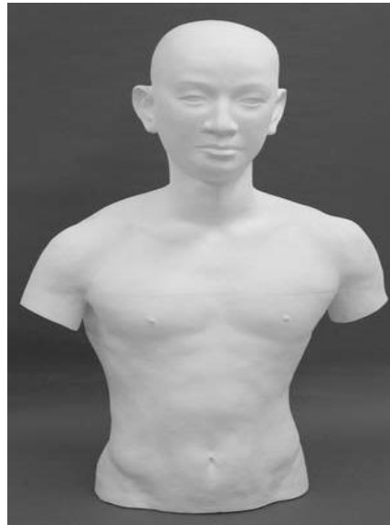
Figure 1.15. Realistic human torso phantom called TYX-151. Source [1]
