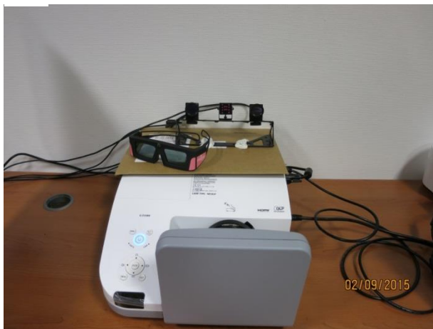
Figure 4.3 a) 3D display platform and eye-tracker. b) The control software of the eye-tracker, the tracking accuracy and head motion are displayed in real time.
