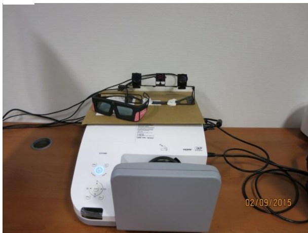
Figure 4.3 a) 3D display platform and eye-tracker. b) The control software of the eye-tracker, the tracking accuracy and head motion are displayed in real time.
