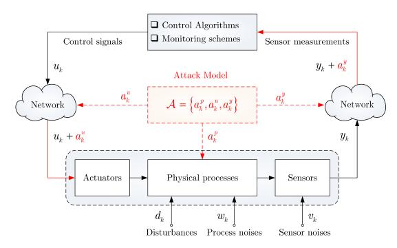
Figure 1.7 – Cyber-physical attacks on SCADA systems: physical attacks on processes (i.e., modeled by physical attack vector  $a_k^p$ ), cyber attacks on control signals (i.e., modeled by control attack vector  $a_k^u$ ), and on sensor measurements (i.e., modeled by sensor attack vector  $a_k^u$ ).
