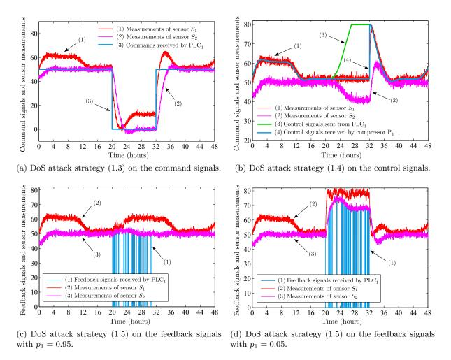
Figure 6.3 – DoS attack strategies on the SCADA gas pipeline.
