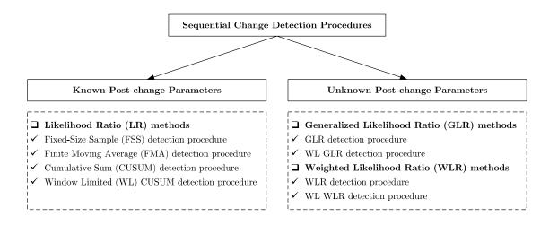
Figure 2.5 – Sequential quickest change detection procedures.
