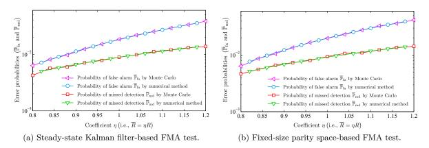
Figure 6.21 – Comparison between the numerical method and the Monte Carlo simulation. The error probabilities ( $\overline{\mathbb{P}}_{fa}$  and  $\overline{\mathbb{P}}_{md}$ ) are described as a function of the coefficient  $\eta$ , where  $\overline{R} = \eta R$ .
