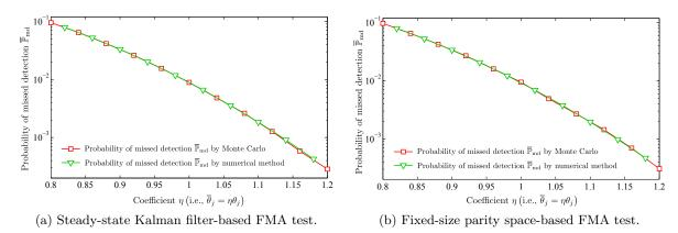
Figure 6.17 – Comparison between the numerical method and the Monte Carlo simulation. The probability of missed detection  $\overline{\mathbb{P}}_{md}$  is described as a function of the coefficient  $\eta$ , where  $\overline{\theta}_j = \eta \theta_j$  for  $1 \leq j \leq L$ .
