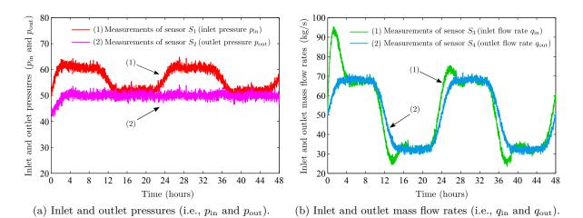
Figure 6.2 – Normal operation of the SCADA gas pipeline.
