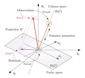
Figure 3.2 – Nuisance parameter rejection by the orthogonal projection of the observations onto the parity space.
