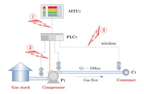
Figure 5.1 – A simple SCADA gas distribution network.
