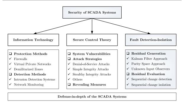
Figure 1.3 – Attack detection and isolation methods.
