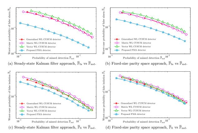
Figure 6.27 – Comparison between the proposed FMA detection rule and the WL CUSUM-based schemes for the scenario 1, i.e.,  $\rho_{12} \ge \max \{\rho_{01}, \rho_{02}\}$ . The worst-case probability of false alarm  $\overline{\mathbb{P}}_{fa}$  and the worst-case probability of false isolation  $\overline{\mathbb{P}}_{fi}$  are described as a function of the probability of missed detection  $\overline{\mathbb{P}}_{md}$ . The change-point  $k_0$  is chosen as  $k_0 = L + 1 = 9$ .
