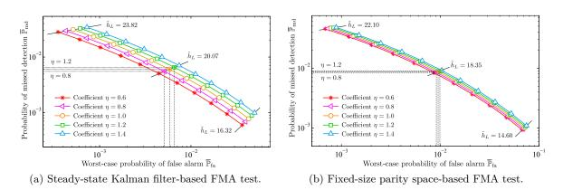
Figure 6.18 – Sensibility of the FMA test with respect to the process noises. The probability of missed detection  $\overline{\mathbb{P}}_{md}$  is described as a function of the worst-case probability of false alarm  $\overline{\mathbb{P}}_{fa}$  for different values of  $\eta = \{0.6, 0.8, 1.0, 1.2, 1, 4\}$ . The true process noise variance is related to its putative value by  $\overline{Q} = \eta Q$ .
