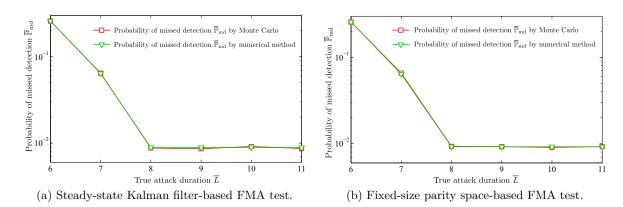
Figure 6.15 – Comparison between the numerical method and Monte Carlo simulation. The probability of missed detection  $\overline{\mathbb{P}}_{md}$  is described as a function of the true attack duration  $\overline{L} = \{6, 7, 8, 9, 10, 11\}$ , for both the Kalman filter approach (left) and the parity space approach (right).
