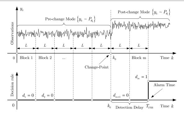
Figure 2.6 – Fixed-size sample (FSS) detection procedure.
