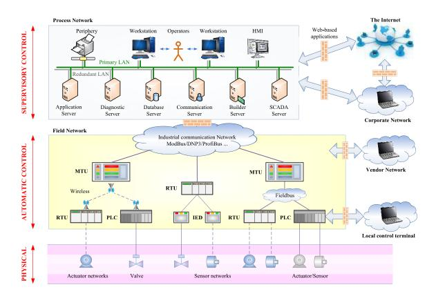
Figure 1.1 – Typical architecture of a modern SCADA system.
