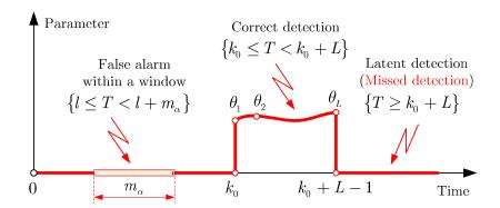
Figure 3.1 – Transient change detection criterion.
