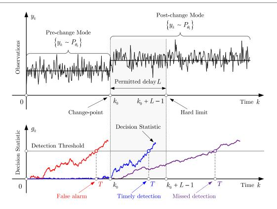
Figure 2.10 – Transient change detection problem for safety-critical applications.
