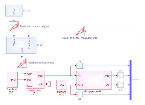
Figure 6.1 – Simulation model of a simple SCADA gas pipeline.
