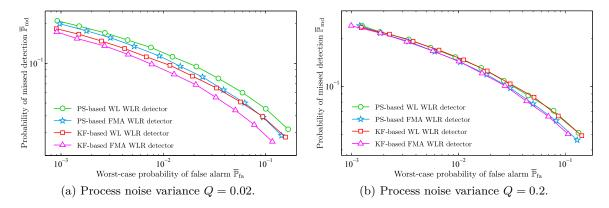
Figure 6.23 – Comparison between the FMA WLR test and the WL WLR test. The probability of missed detection  $\overline{\mathbb{P}}_{md}$  is described as a function of the worst-case probability of false alarm  $\overline{\mathbb{P}}_{fa}$ . The *a priori* distribution of the parameter  $\gamma$  is chosen as  $\gamma \sim \mathcal{U}(0.5, 1.5)$ .
