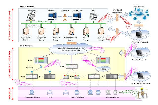
Figure 1.2 – Possible attack points to modern SCADA systems.
