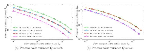
Figure 6.22 – Comparison between the FMA GLR test and the WL GLR test. The probability of missed detection  $\overline{\mathbb{P}}_{md}$  is described as a function of the worst-case probability of false alarm  $\overline{\mathbb{P}}_{fa}$ .
