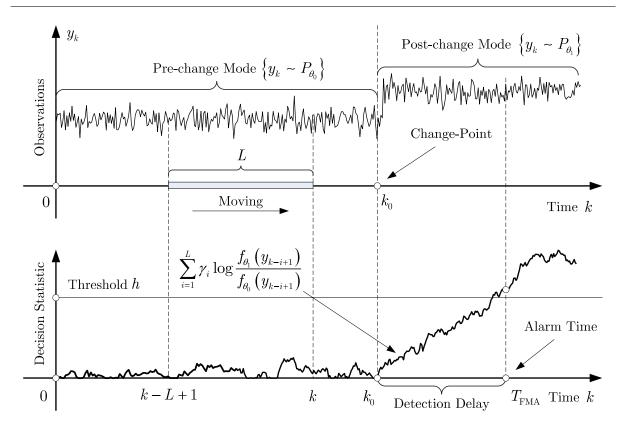
Figure 2.7 – Finite moving average (FMA) detection procedure.
