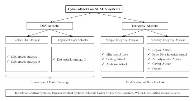
Figure 1.5 – Classification of cyber attacks on SCADA systems.
