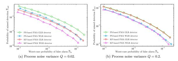
Figure 6.24 – Comparison between the FMA GLR test and the FMA WLR test for Q = 0.02 and Q = 0.2. The parameter  $\gamma$  is fixed at value  $\gamma = 1$  for the WLR-based detectors.
