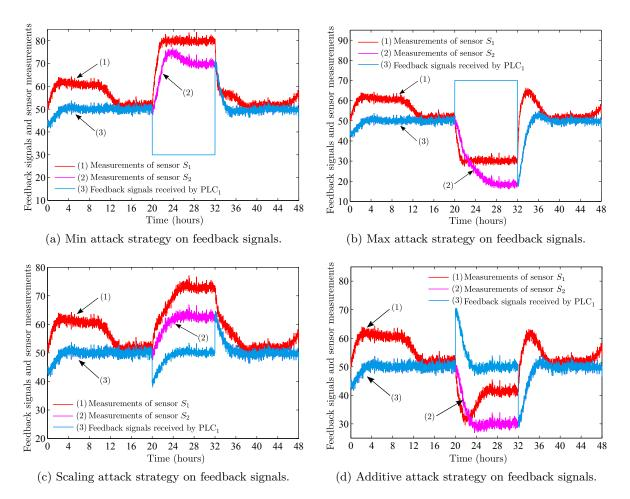
Figure 6.6 – Simple integrity attacks on feedback signals transmitted from sensor  $S_2$  to the PLC<sub>1</sub>.
