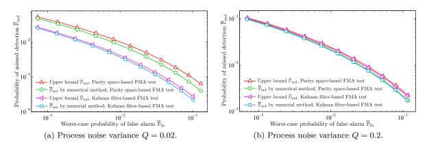
Figure 6.9 – Upper bound  $\tilde{\mathbb{P}}_{md}$  for the worst-case probability of missed detection  $\overline{\mathbb{P}}_{md}$  of the FMA detector. The simulation has been performed with the process noise variances Q = 0.02 and Q = 0.2, respectively. The change-point for the numerical method is chosen as  $k_0 = L + 1 = 9$ .
