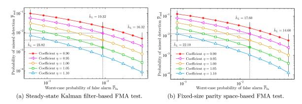
Figure 6.16 – Sensitivity of the FMA test with respect to the attack profiles. The probability of missed detection  $\overline{\mathbb{P}}_{md}$  is described as a function of the worst-case probability of false alarm  $\overline{\mathbb{P}}_{fa}$  for different values of  $\eta = \{0.90, 0.95, 1.00, 1.05, 1.10\}$ . The true attack profiles are related to the putative attack profiles by  $\overline{\theta}_j = \eta \theta_j$ , for  $1 \leq j \leq L$ .
