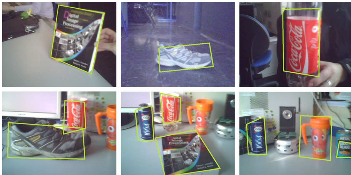
Fig. 12 Camera pictures from single ( first row ) object detection and multiple ( second row ) previously learned object detection
