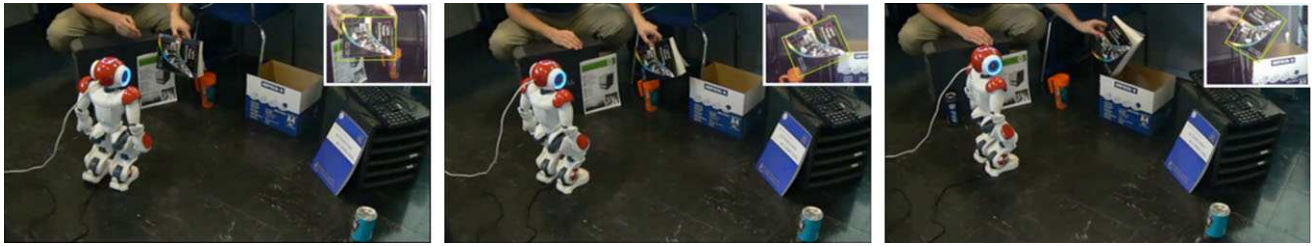
Fig. 11 Images from tracking a previously learned moving object. Robot camera picture is shown in upper right corner of each image
