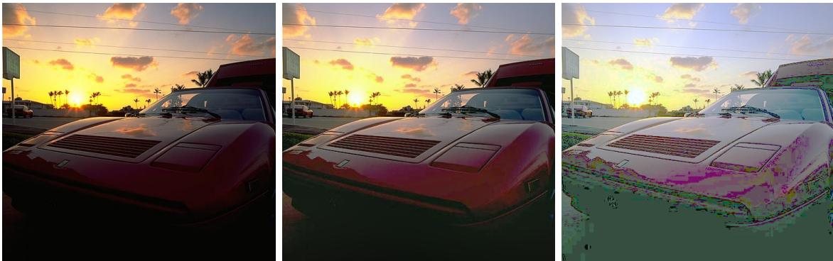
Figure 1.3: Left : original image. Center : color enhancement obtained via gradient descent minimization of a perceptual functional. Right : effect of histogram equalization. Image courtesy of Peter Greenspun.
