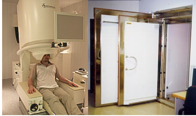
Figure 3.4.: From left to right, research participant with MEG instrument and an entrance to a magnetically shielded room, showing the separate shielding layers.
