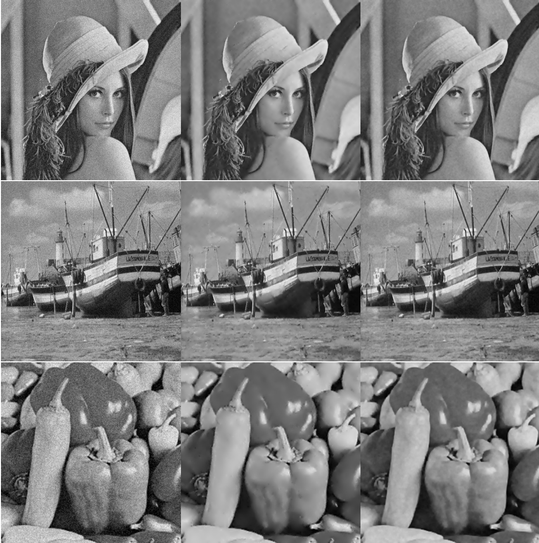
Figure 1.20.: From left to right, the noisy image ( \sigma = 15 ), the reconstructions with respectively Bai and Feng's algorithm [24] and Algorithm 3, the fractional order \alpha is equal to 1.5. From top to bottom, the Lena image, the Boat image and the Peppers image.
