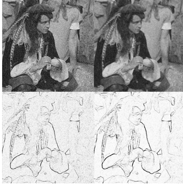
Figure 1.6.: From left to right, first line noisy Man image ( \sigma = 0.12 ), solution of Equation (1.3), second line, lowest eigenvalues of M_{MS}(x) (1.36), lowest eigenvalues of M(x) (1.17).
