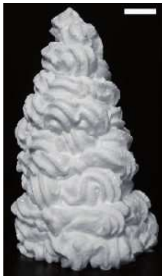
Figure 1.5: An aqueous foam stabilized by silica nanoparticles. Scale bar is 1 cm
